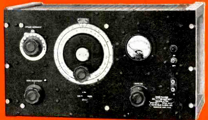
Left to Right, TOP: Frequency increment dial—main frequency control—output voltmeter. BELOW: Zero adjustment—range switch—output control.
