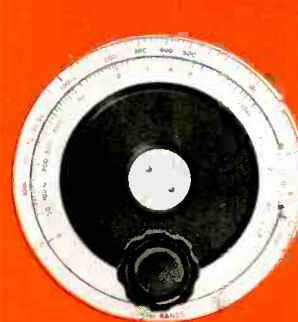
Main frequency dial engraved approximately logarithmically—scale length per decade 3\frac{1}{2} inches.
