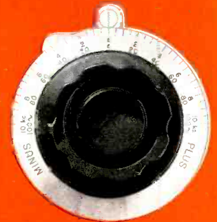
Frequency increment dial—plus or minus: 100 cycles, low range; plus or minus 10 kilocycles, high range.
