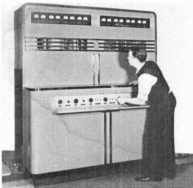
The new RCA 1 kw. television transmitter. It is believed that the power of this transmitter is sufficient to enable experimental stations to render a satisfactory service over a reasonable area.
