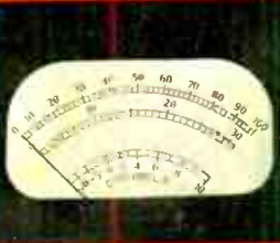
Illuminated linear meter with auxiliary db scale
