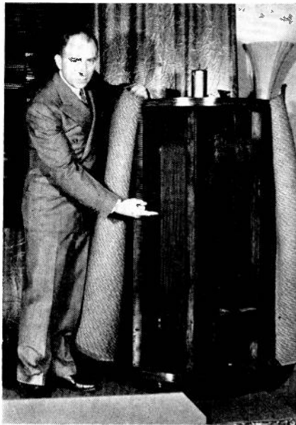
P. F. Hadlock demonstrating a jumbo model of the G-E Beamscope. The rejector shield has been torn back to show windings.
