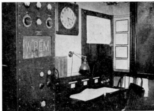
Fig. 1 Transmitter at left. Center on desk radio receivers. Speakers shown at right.
