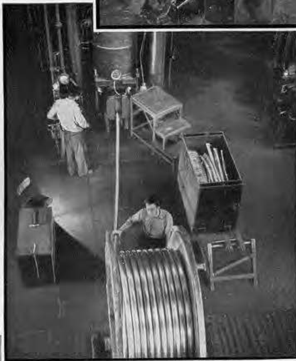
These machines saturate wire insulation with asphaltic materials for protection against the elements.
