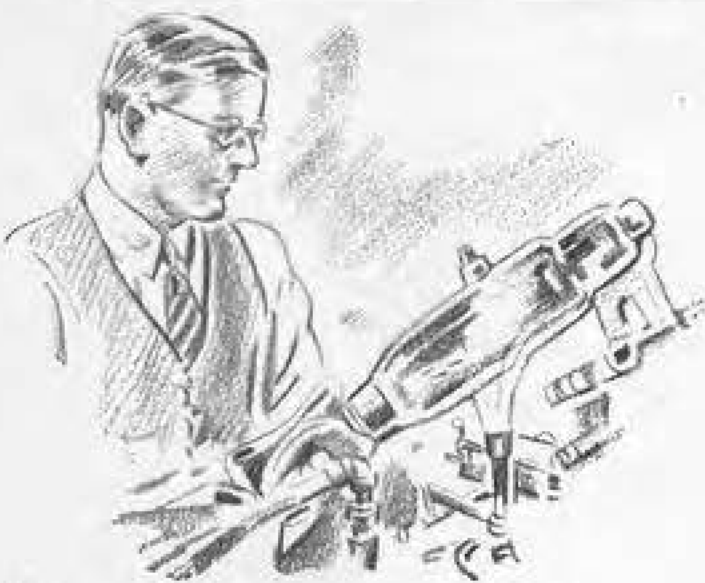
Vacuum tubes gently treated to prevent cracking.
