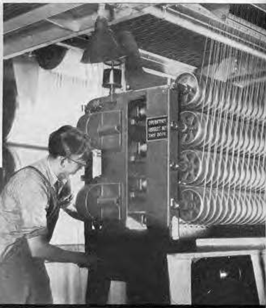
Makes paper insulation on 60 wires at once.
