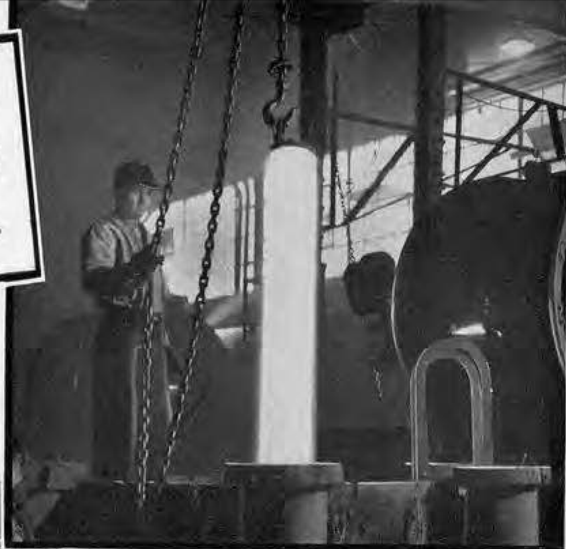
...casting a bronze billet from salvaged material Nassau Smelting and Refining Company.
