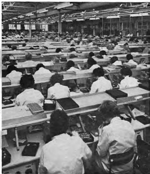
Assembling MAZDA valves at the Rochester factory.
