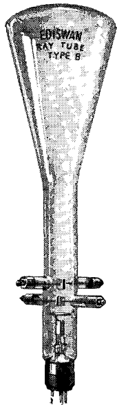
EDISWAN Type B 4 in. gas focused electrostatic tube first produced in 1930.
