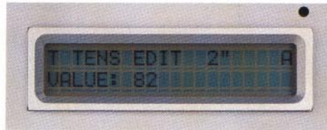
Example: Indication of tape tension setting for EDIT/2" tape, tape type A
