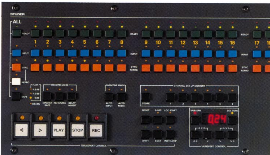
The audio remote control unit with tape transport keys, channel status memory, varispeed and other enhanced functions.
