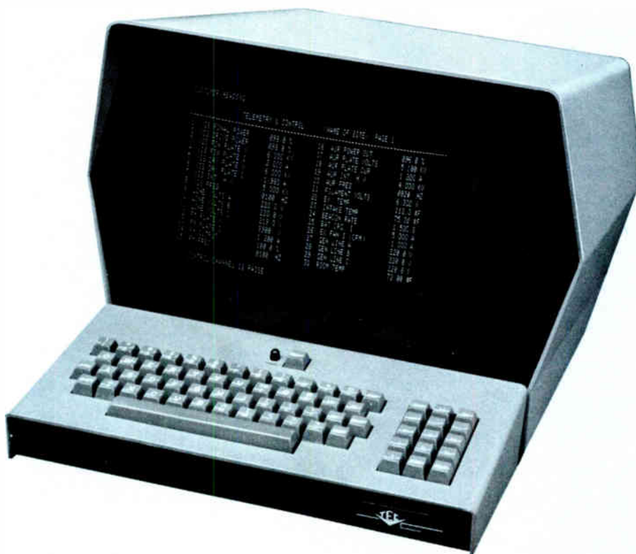
Optional Video Reader. Connects to Central Processing Unit at studio site and includes command capability through keyboard.
