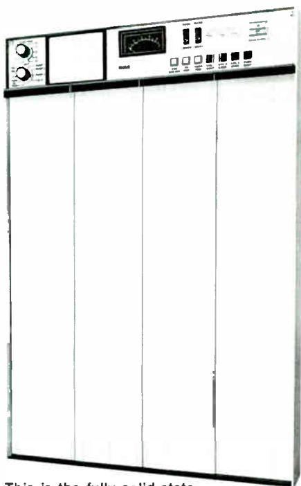
This is the fully solid-state exciter/modulator unit.
