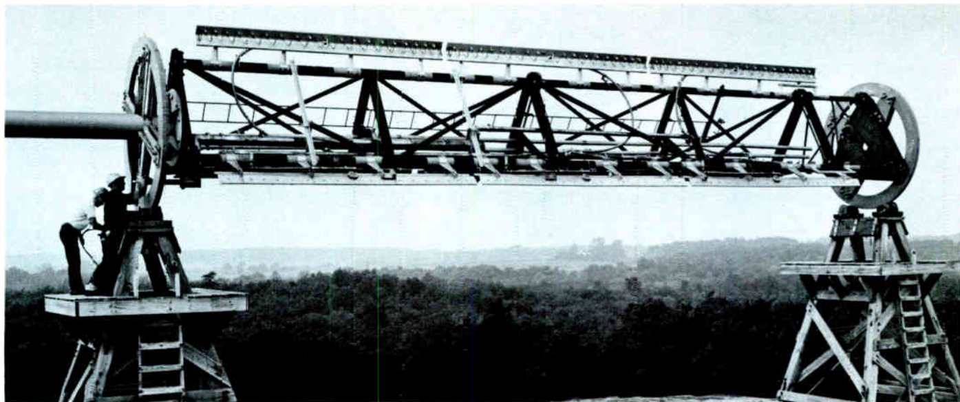
A three-layer Vee-Zee array undergoing pattern tests.
