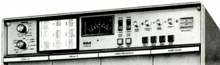
Exciter/modulator control panel.
