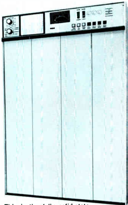
This is the fully solid-state exciter/modulator unit.
