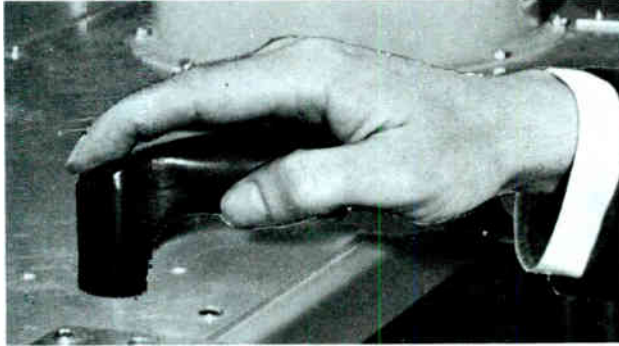
Built-in switch disconnects individual power amplifier cubicle from operating transmitter.
