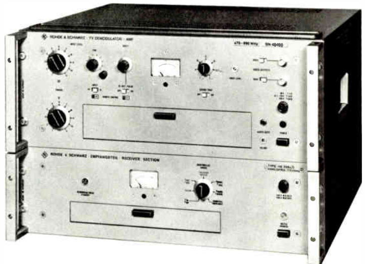
For off-air use of the demodulator, a receiver unit is available. It is the lower unit in this photo.
