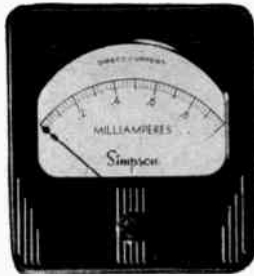
MODELS 27, 37, 47, 57 3 1/2" RECTANGULAR CASE. Width, 3"; height, 3 1/4". Mounts in round hole. Body diameter, 2 3/4". Scale length, 2-9/16". Bakelite case.
