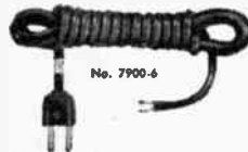
REPLACEMENT CORD WITH MOLDED VINYL CAP — BARE ENDS FOR LAMPS, EXTENSION CORDS, RADIOS, RECORD PLAYERS, TV, SMALL APPLIANCES, CLOCKS, ETC. Made of UL Approved No. 18 Type S.P.T.-1 (POT) Plastic Wire with Molded Vinyl Cap. Blank End Has 3/4" Strip Ready for Wiring. Each Cord Set Individually Banded.
