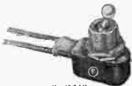
No. 1886-LN TOGGLE CANOPY SWITCH U. S. Navy Approved Type Navy Dwg No. 9-S-5293 Alt. 11 Navy Stock No. A17-S-27001 3/16" Diameter—1/2" Long Nipple 3A.-125V [F] 6A.-125V.—3A.-250V.
