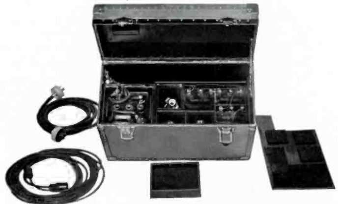
The battery case is equipped with a convenient tray where the cables may be carried, and space is also provided for microphones.
