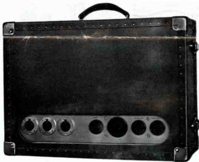
Rear view of the Amplifier-Control Case, showing convenient location of the flush outlet receptacles.
