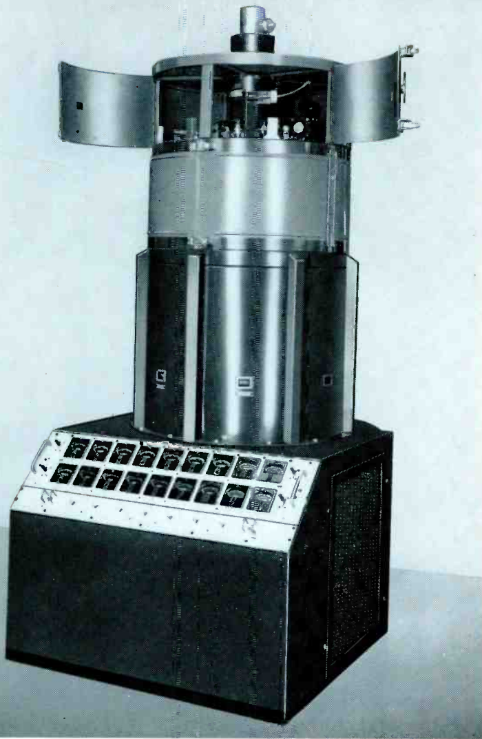
External view of the high band amplifier for channels 7 to 13.
