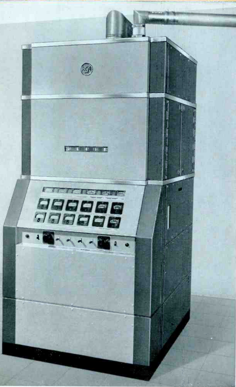
One of the power amplifiers of the TT-100AH showing front panel with tuning motor switches, individual tube meters, tuning indicators, switches and status lamps. Tubes, located behind hinged access doors, are of plug-in type for rapid change.
