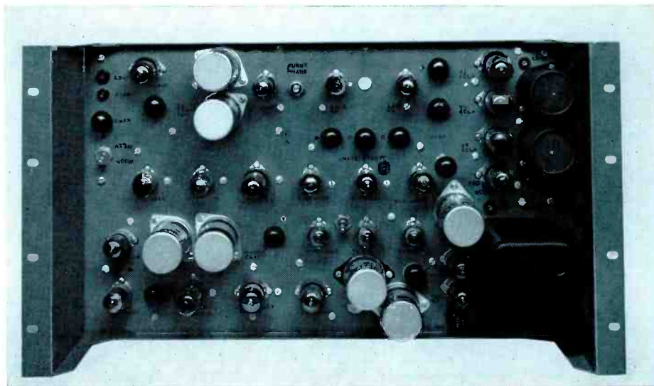
Top view of chassis of the Type TA-7A Stabilizing Amplifier.
