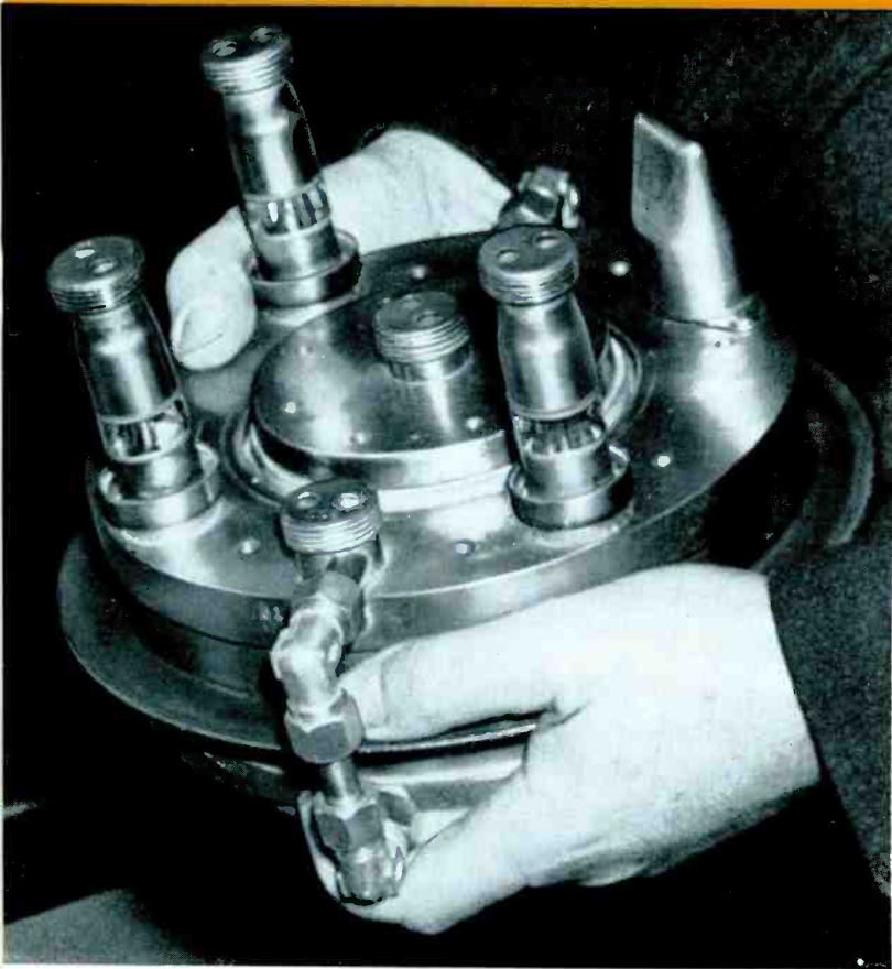
Small-size, conventional tetrodes (RCA Type 6448) are used in the Aural and Visual "P.A." sections of the 12½ KW transmitter. Use of conventional types of tubes throughout results in economical operation, easy maintenance, and simple, straightforward circuitry.
