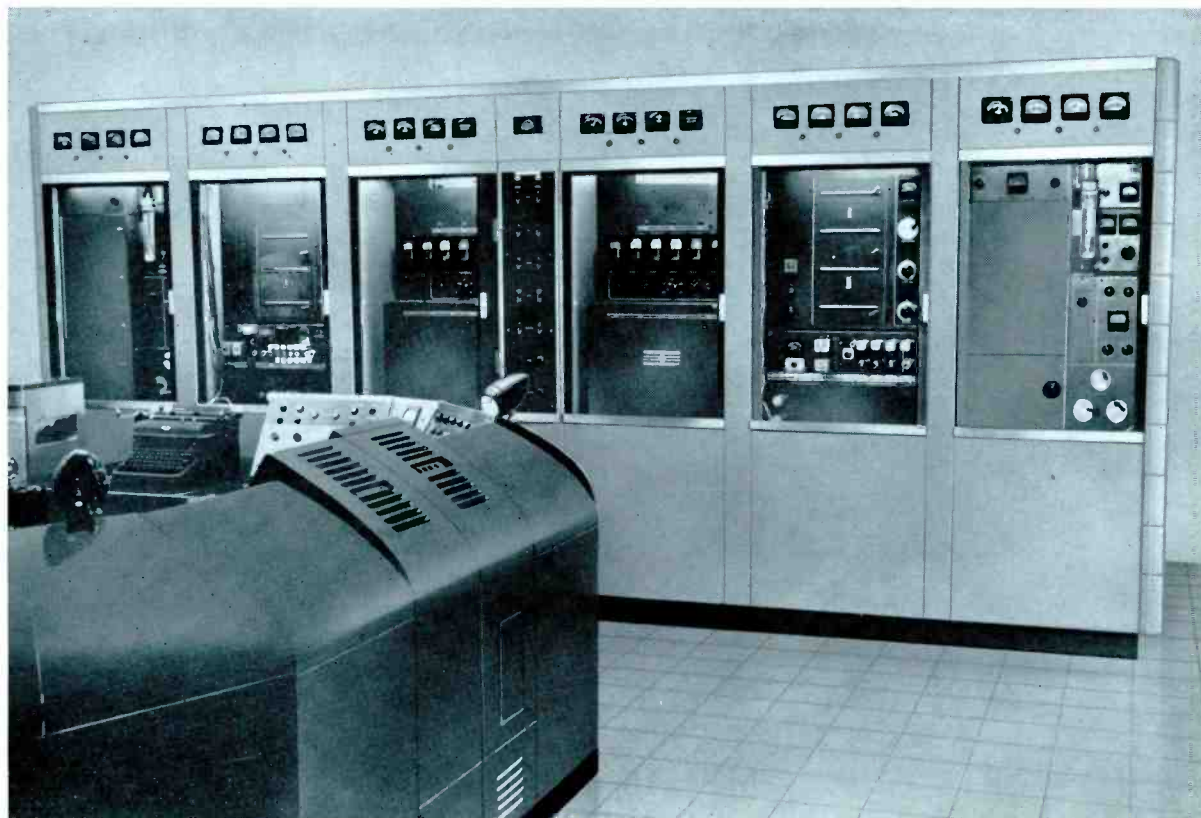
Front view of the TT-10AL/AH with sliding panel doors open. All tubes and other components are easily accessible through front and rear doors.
