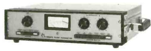
Moseley RPL transmitter and receiver (below), RPL-3 or RPL-4. Identical in appearance, the two Moseley RPL transmitters are available for the 148-174 and 450-470 MHz bands. Equipped with two low-level inputs.
