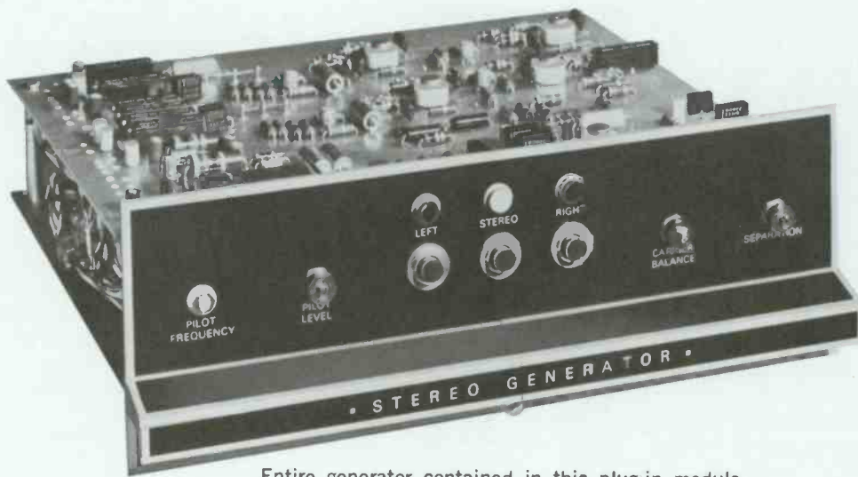
Entire generator contained in this plug-in module.
