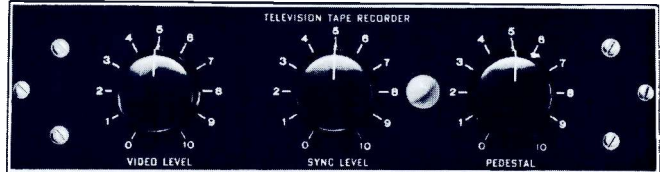
Remote Control Panel (Signal), MI-40692-A
