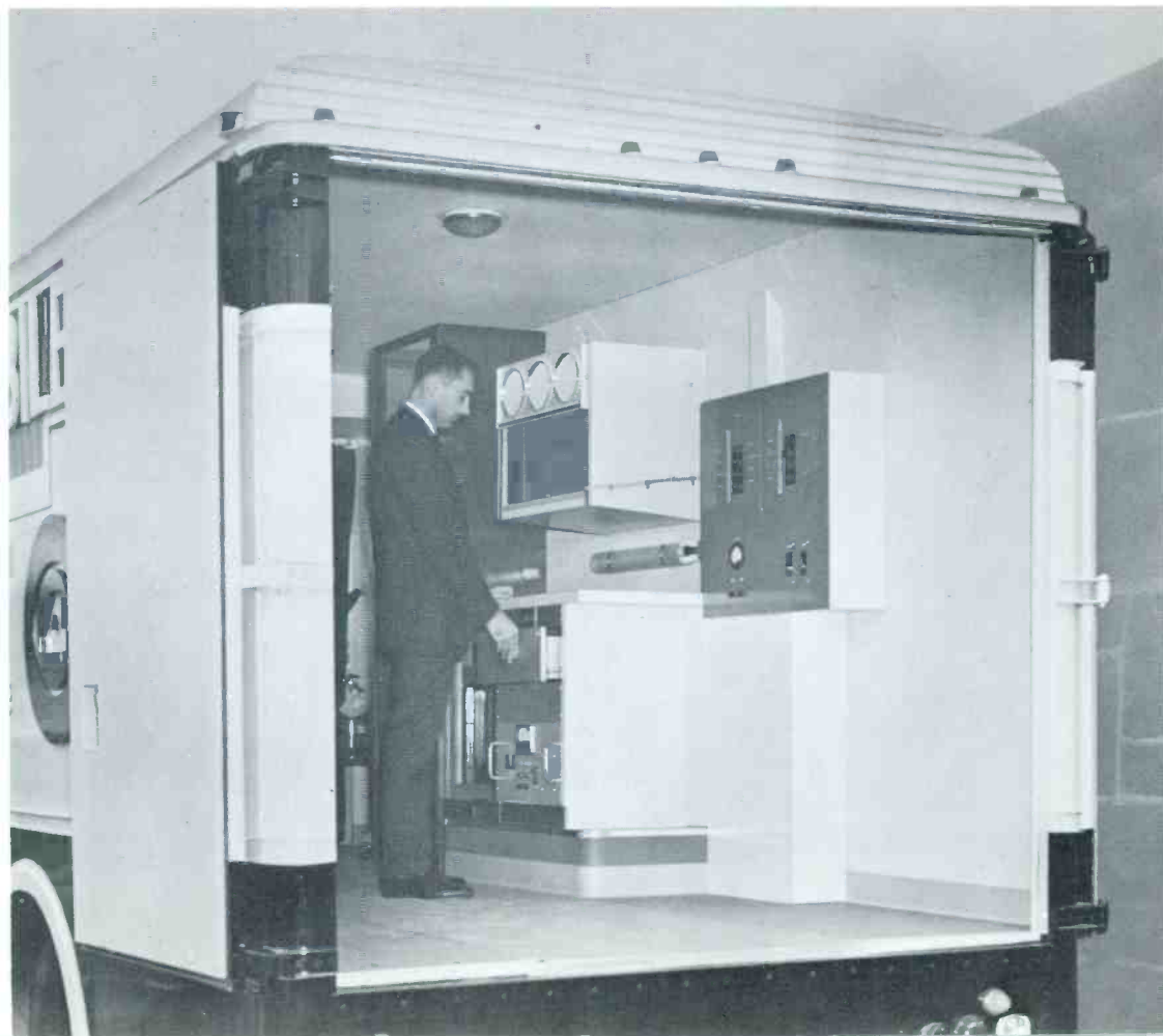
MOBILE TV TAPE RECORDING CENTER —Interior view of TJ-72 showing roomy interior with mounted TR-22 Tape Recorder together with audio facilities, cabinets, and compartments for tape storage, etc. More than 5½ feet of extra space at rear can accommodate field camera chain or other needed equipment for on-location tape recordings.
