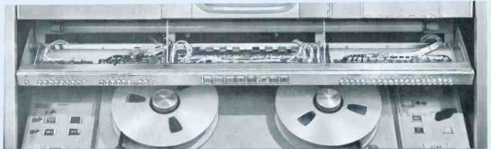
Slide-out switcher panel and components.
