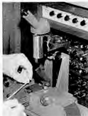
(H) Operator dispensing splicing tape and preparing to place it into proper position.
