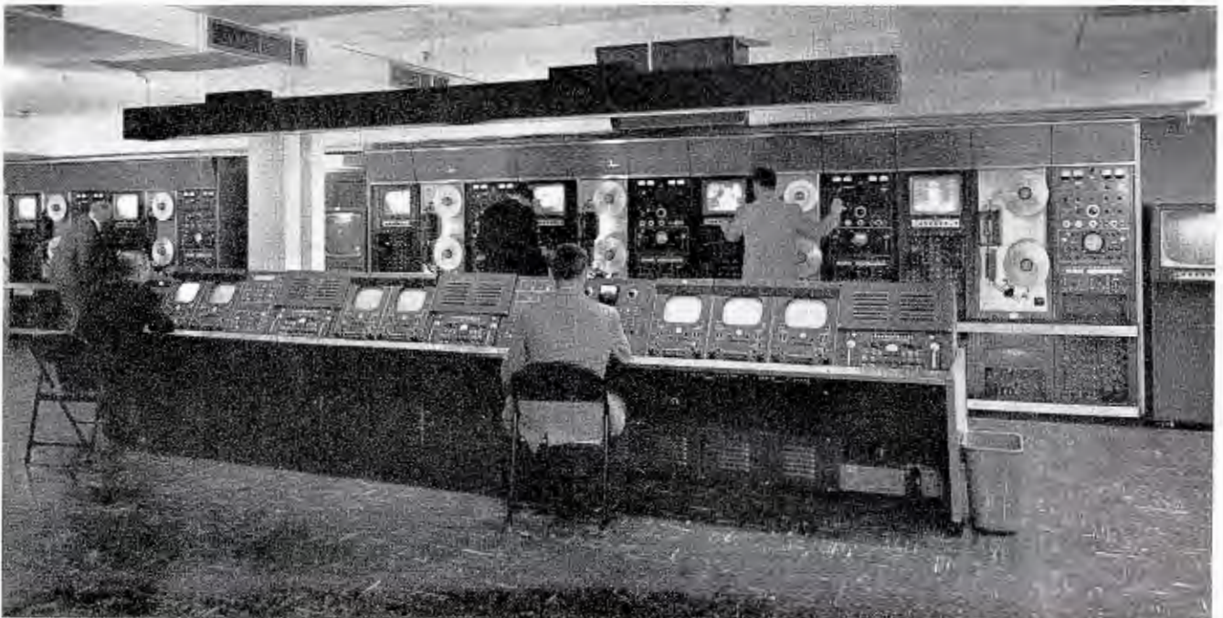
Convenient rack-mounted design permits installation of tv tape recorders with minimum floor space and maximum accessibility.
