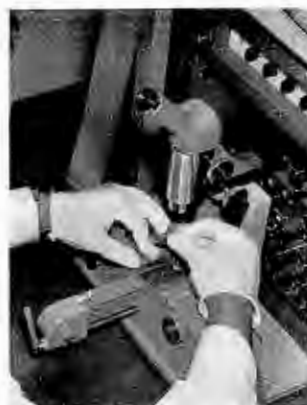
(G) Tape containing the new information is sheared and readied for joining to tape already in splicer.
