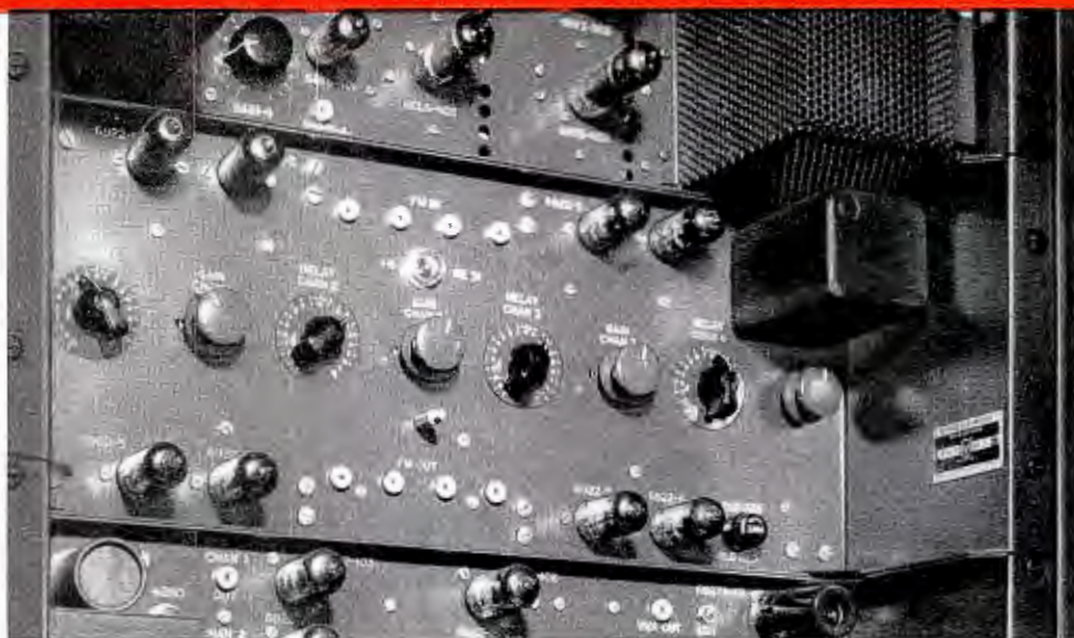
This single chassis is used for manual control of both record and playback quadrature correction in the TR-11. A switch, mounted on the back of the chassis, allows the operator to select playback or record mode.
