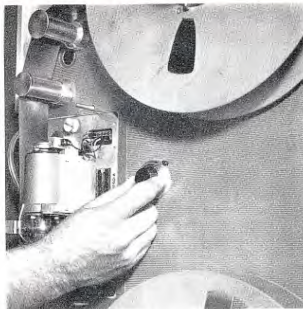
Mechanical adjustment of vacuum guide position is accomplished by vernier calibrated dial as shown above.
