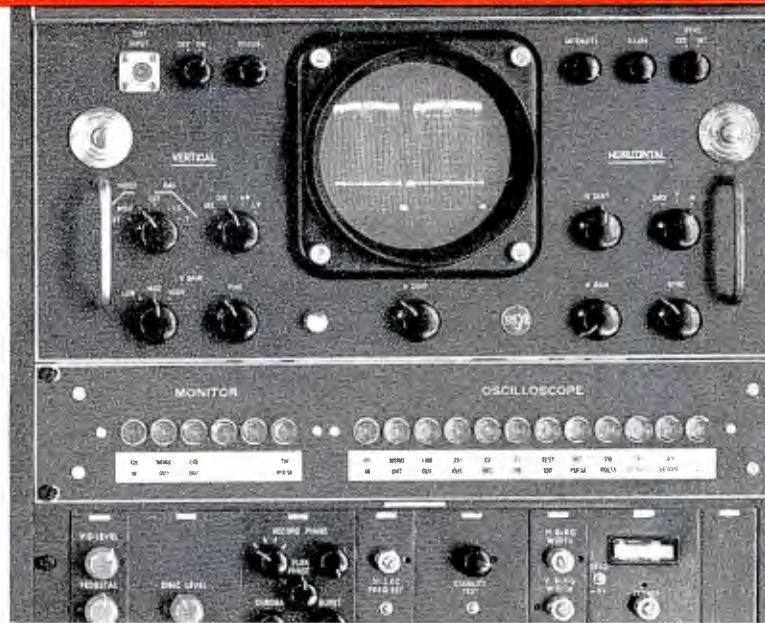
Oscilloscope provides operator with quick check of machine performance. Has built in switching facilities.
