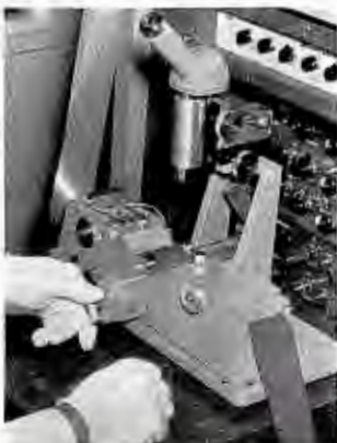
(I) Splicing tape is inserted beneath the lifted ends of the two tapes to be joined.
