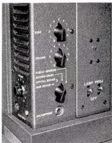
Operating controls are "TONE" and "VOLUME" controls, "MICROPHONE" input, projection "LAMP" and "PROJ" (projector) starting switch. Mixer "VOLUME" control and two "MIXER INPUTS" are mounted adjacent to the rear.
