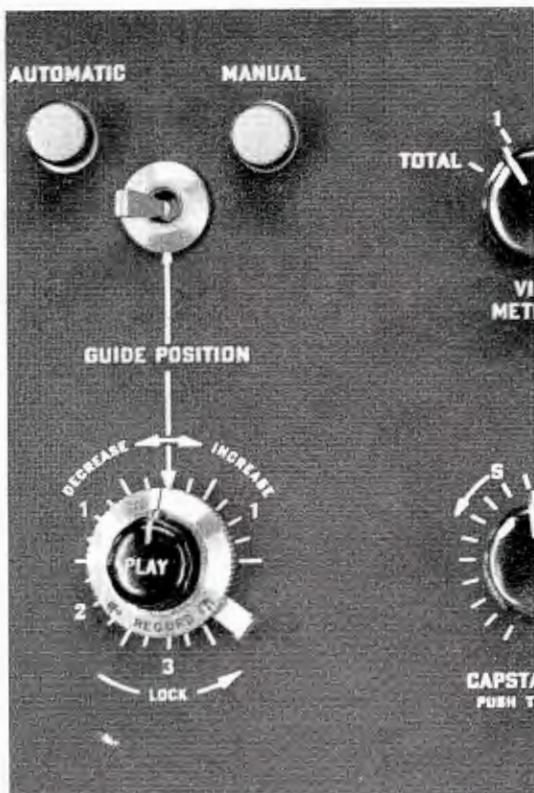
Separate play-record, guide-position controls minimize operator errors.
