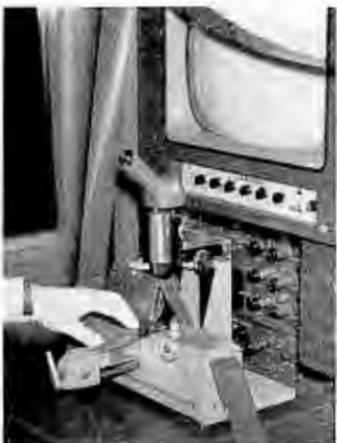
(E) Tape from top supply reel is draped over tape support post and positioned under left hold-down door.
