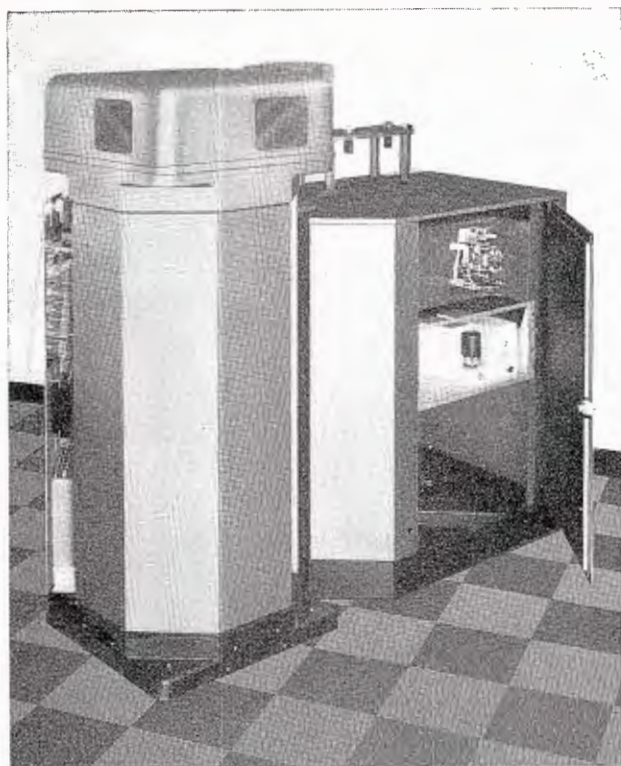
Accessibility of control panel and associated circuits for servicing and large storage cabinet in pedestal are features of TP-15 Universal Multiplexer. Shelf space in pedestal is equivalent to 3 feet of standard rack space.
