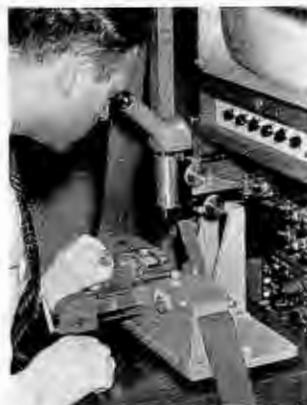
(F) Aligning the tape track prior to making the precision cut.
