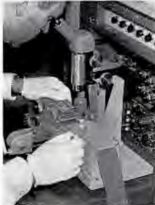
(C) Operator aligns edge of video track on the built-in reticule in order to cut tape halfway between adjacent video tracks.
