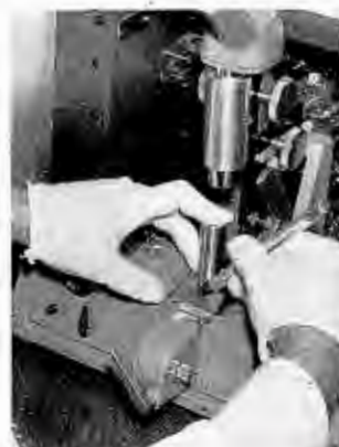
(K) Excess splicing tape is trimmed by means of trimming tools.
