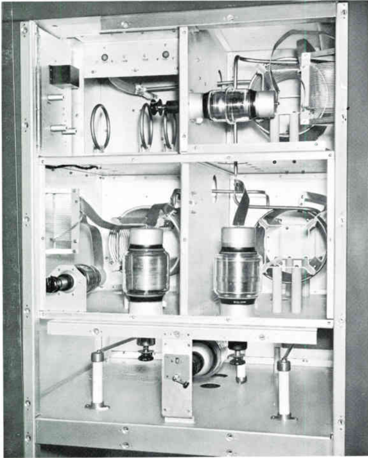
Upper rear of exciter portion of the BTA-50J showing the combining and output networks.
