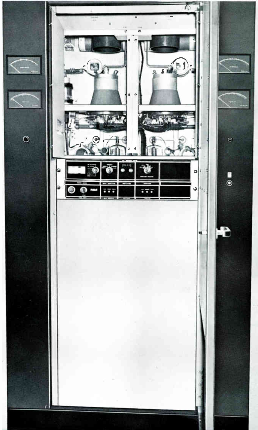
Front section of the exciter-modulator containing all components from oscillator through the driver stages.
