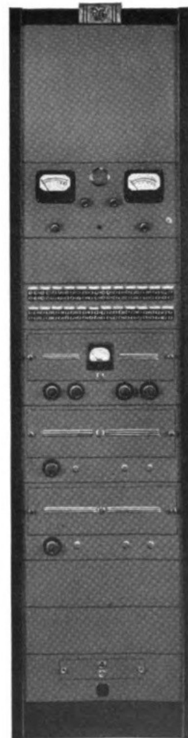
MI-11620-F Transmitter Monitor and Amplifier Rack as shipped.
