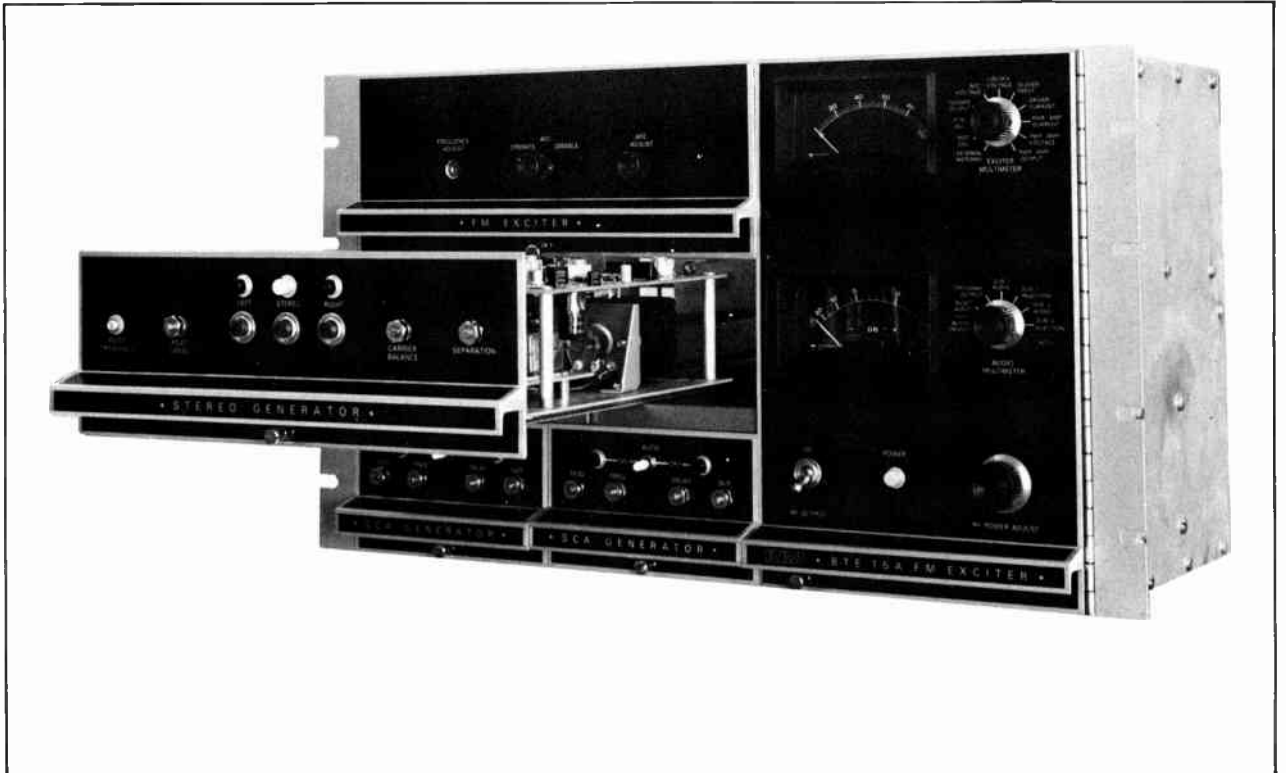
Figure 8. BTE-15A System, Module Extender Installed
