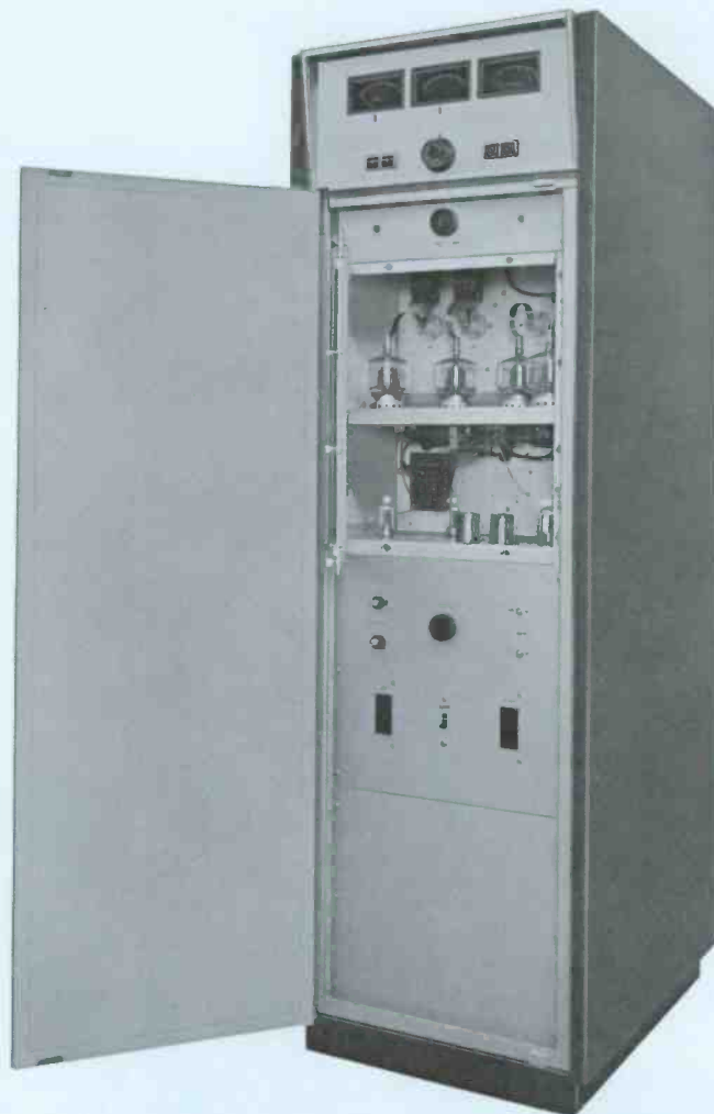
Type BTA-1S Transmitter with outer and inner door open to display accessibility to the tubes. Power amplifier and modulator tubes are near top while the lower chassis carries the audio-amplifier and intermediate stages.
