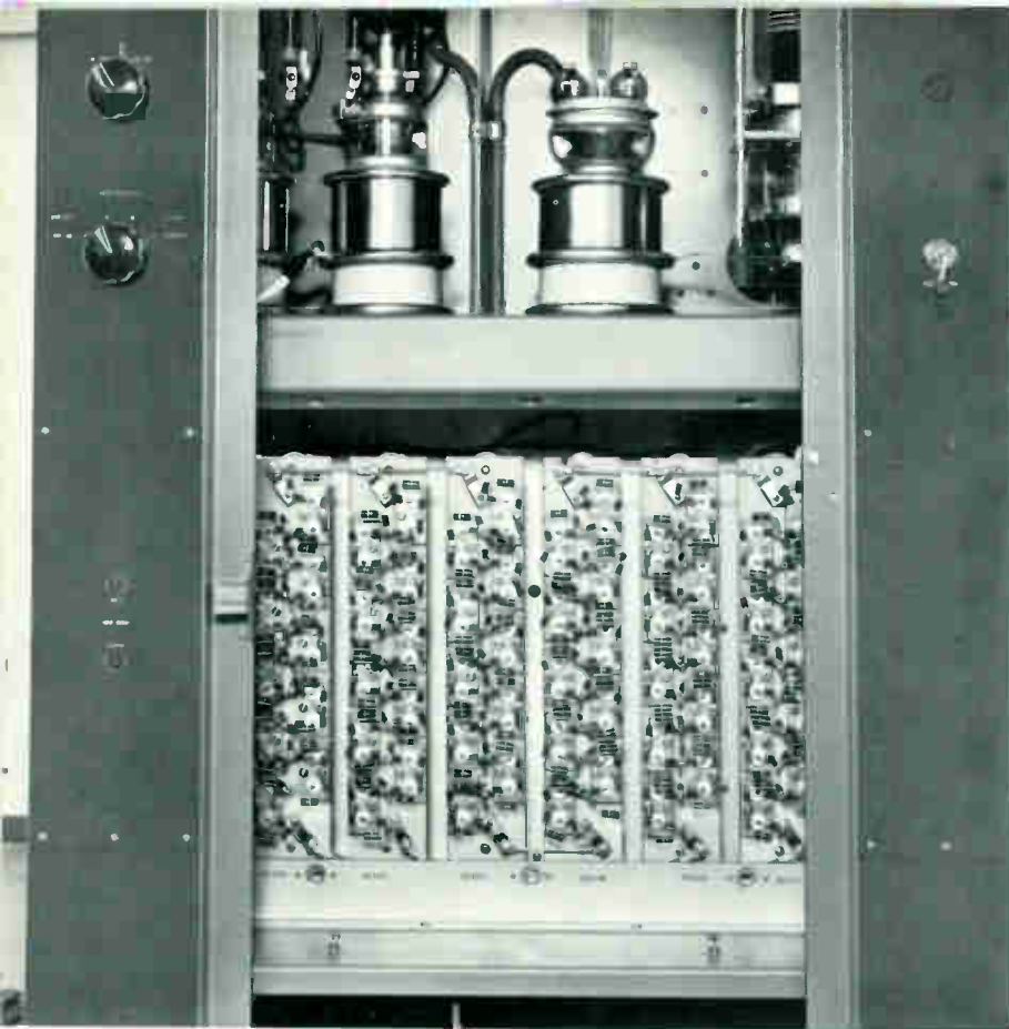
Front view of the Silicon Rectifier Chassis of the BTA-5T1. The silicon cells offer improved performance since they are particularly resistant to aging, moisture and wide temperature variations.
