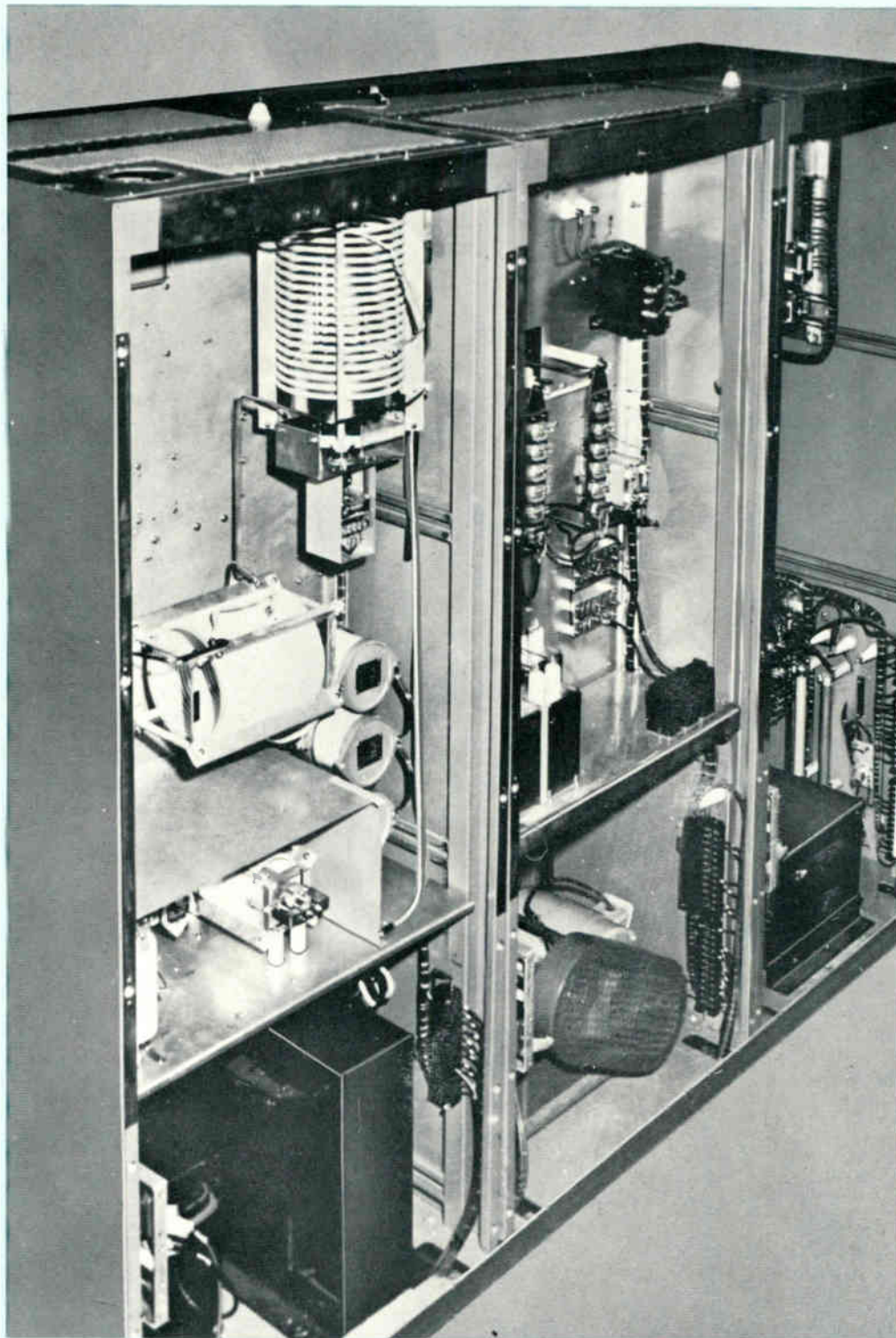
Rear view of transmitter showing vertical construction permitting complete accessibility to all transmitter facilities. The modulation transformer and final PA tank circuitry are seen in foreground, rear of modulator and blower in center cabinet, while heavier components of driver are shown mounted on floor of third cabinet.
