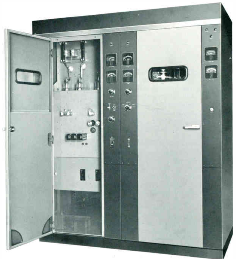
IPA and modulator driver stages of the BTA-5T1 can be seen at top of open cabinet. The exciter is at the center of the cabinet, and control equipment is placed just below the exciter
