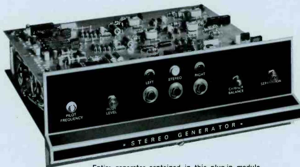
Entire generator contained in this plug-in module.
