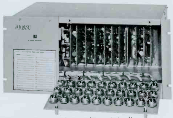
Fold-down front panel in transmitter-control unit provides quick access to all modules. Note 10-turn potentiometers on panel.
