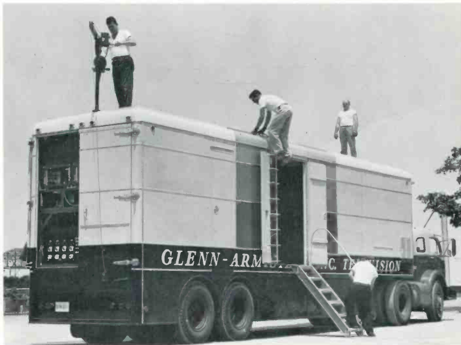
Standard 35-foot trailers with custom body built to be structurally sound and equipped for TV production requirements offer maximum mobile facilities. TJ-90 design includes king pin trailer hitch, air brakes, under floor wiring trench, ceiling tie bars for equipment support, heavy-duty floor covering, insulated walls and ceiling, special access doors, curbside door ladder, compartmentalized construction to house each unit of TV equipment and many other plus features.
