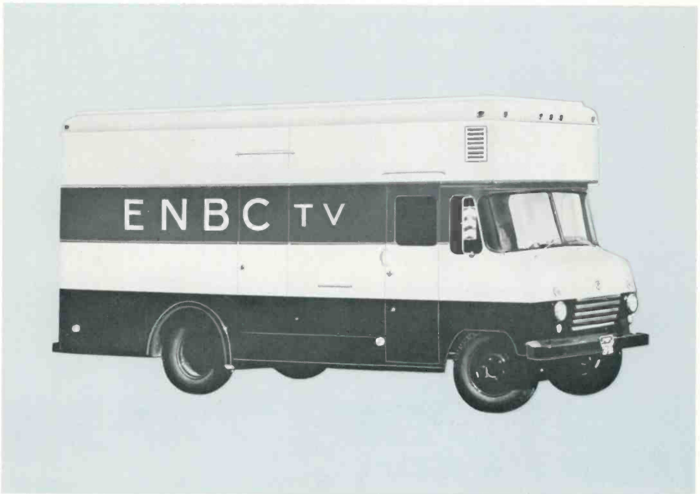
Typical of the RCA Mobile Truck is the TJ-70 pictured. Maximum equipment storage space underside, balanced weight distribution, and air conditioning with cooling and heating units are design considerations. Featured is a fiberglass front with curved windshields and the central air conditioner mounted above the cab.
