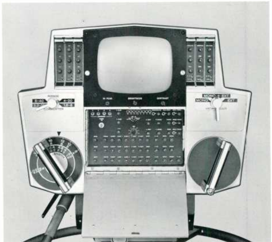
TK-42 Camera showing conveniently located set-up control panel.
