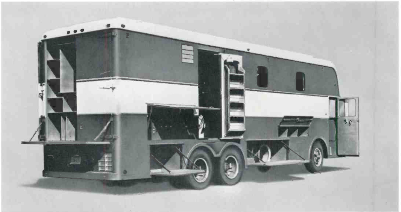
An RCA custom bus design illustrating maximum utilization of all available space for equipment storage.
