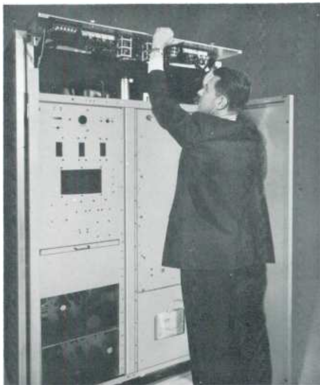
EASE OF MAINTENANCE —Full access to all transmitter sections is an important feature in the mechanical design of the BTF-20E.
