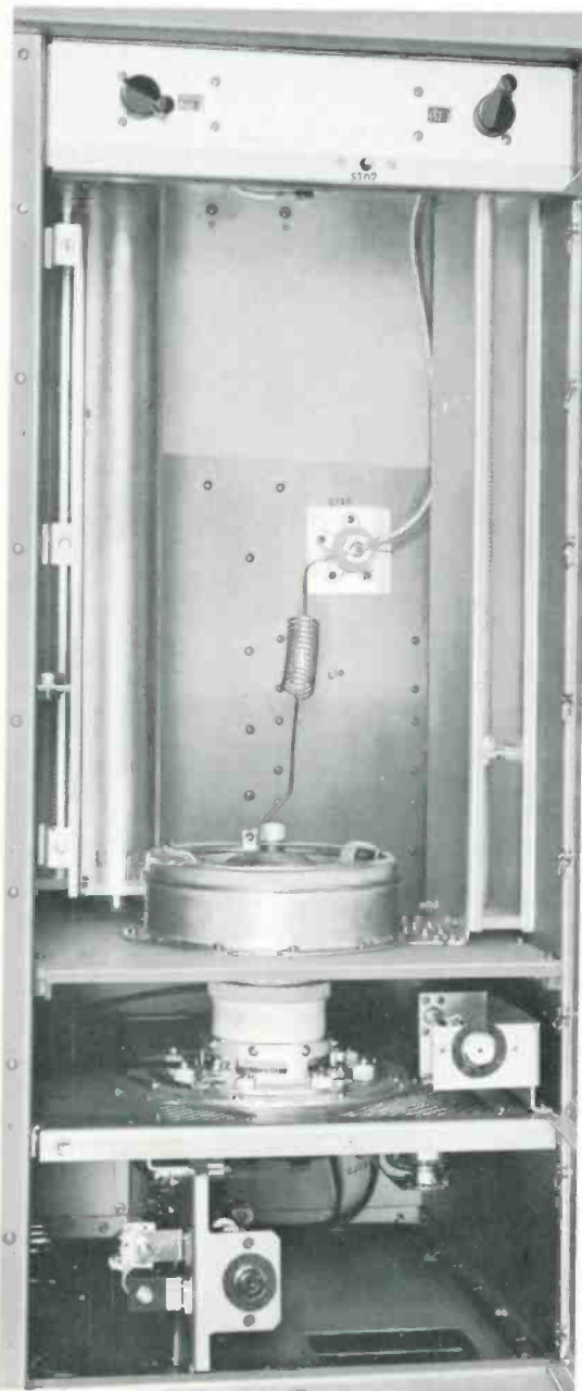
ONLY TWO TUBES BETWEEN EXCITER AND OUTPUT —View showing interior of PA and IPA cabinet with the 4CX10000A ceramic tetrode and one 7203/4CX250B IPA tube below shelf. These supply the necessary power for the full fidelity BTF-10E.
