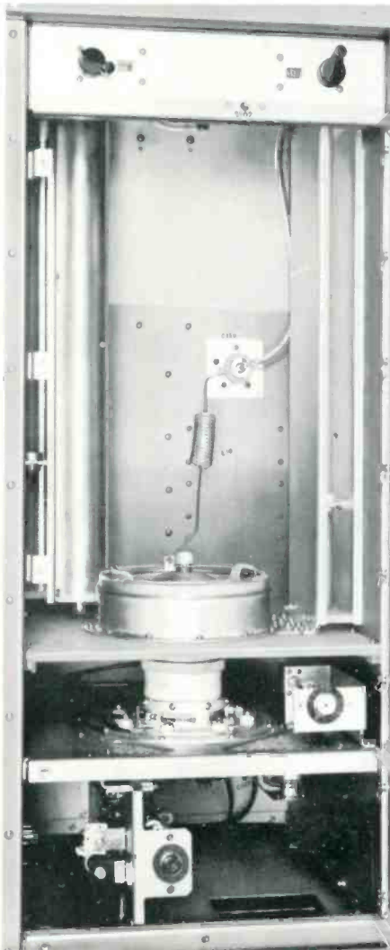
ONLY TWO TUBES BETWEEN EXCITER AND OUTPUT —View showing interior of PA and IPA cabinet with the 4CX5000A ceramic tetrode and one 7203/4CX250B IPA tube below shelf.
