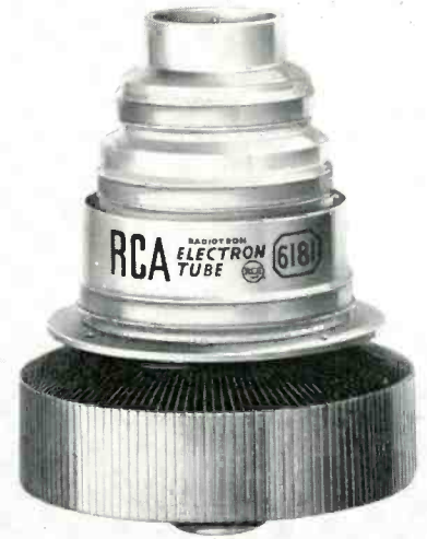
FIG. 12. 6181 tube used in both aural and visual outputs.
