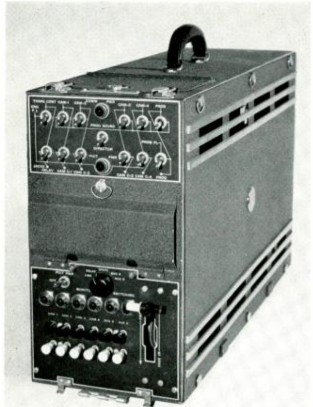
FIG. 2. Field Switching System.
