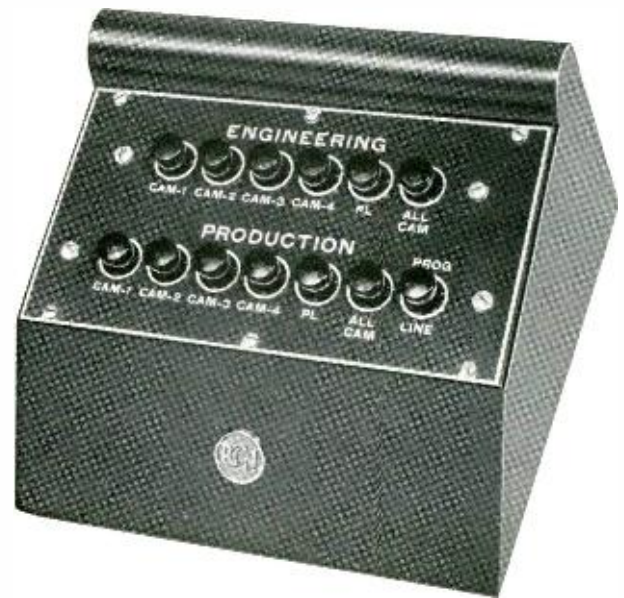
FIG. 5. View of the "Intercom" control box which contains two banks of pushbuttons for engineering and production personnel.
