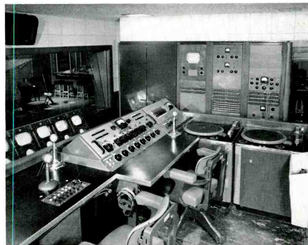
FIG. 22. View of a television studio control room showing video and audio monitoring facilities.
