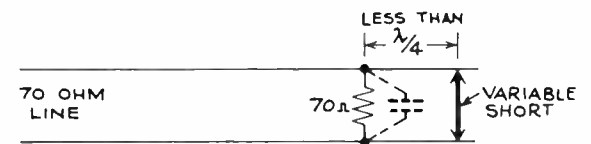
"B" - INDUCTIVE SECTION ADDED AND RESONATED WITH CAPACITY TO THE INPUT FREQUENCY.
