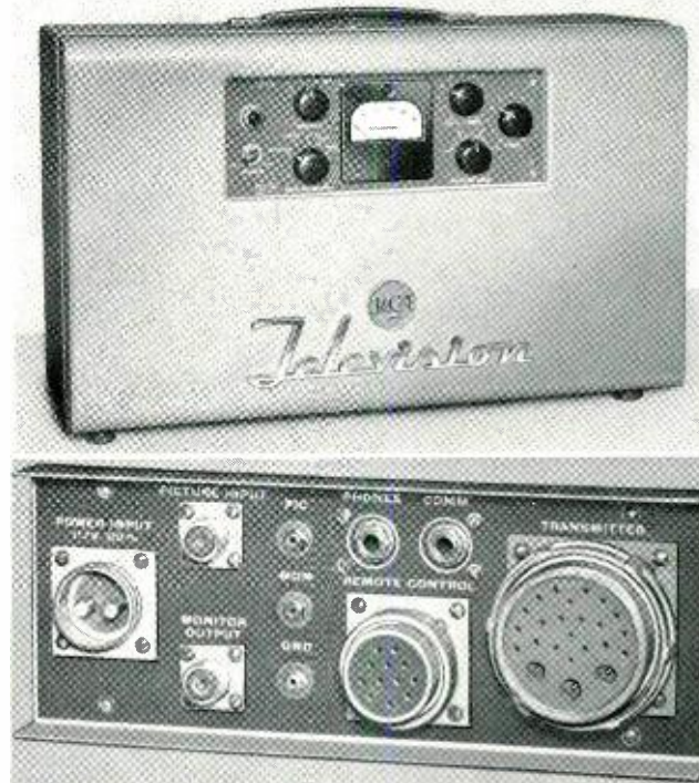
FIG. 5. View of transmitter control unit and close-up of connection panel for the TTR-1B.
