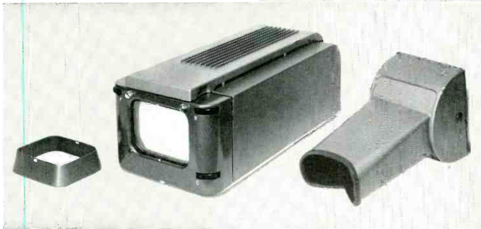
FIG. 14. Viewfinder opened up to show accessibility to 7" Kinescope and components. ▶
