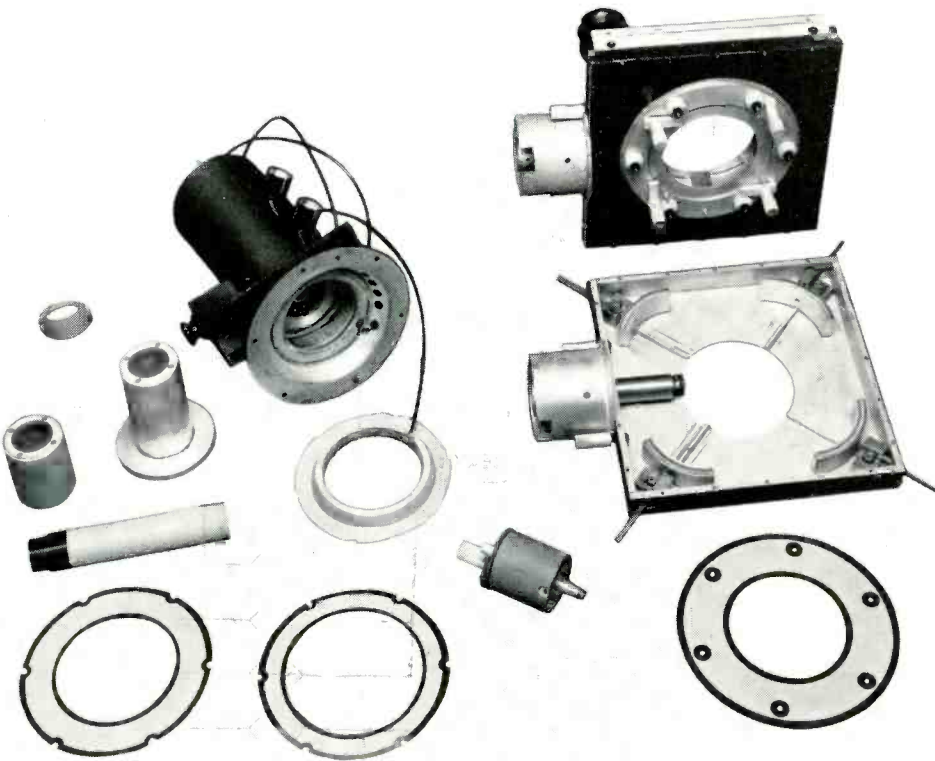
FIG. 11. PA cavity completely disassembled.
