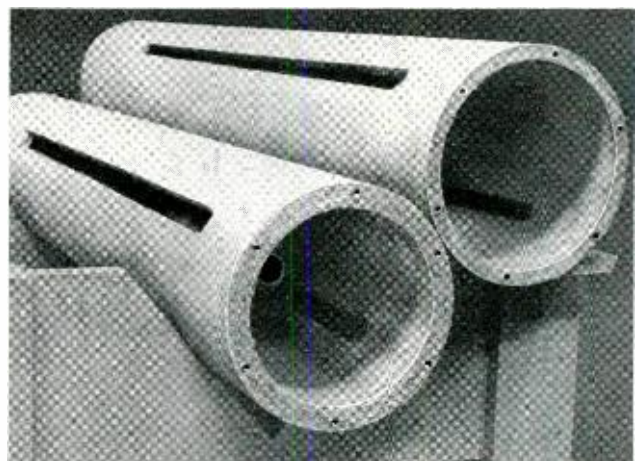
FIG. 4. View showing difference between normal 8-inch pipe and pipe used for 75/47 lb. windloading.
