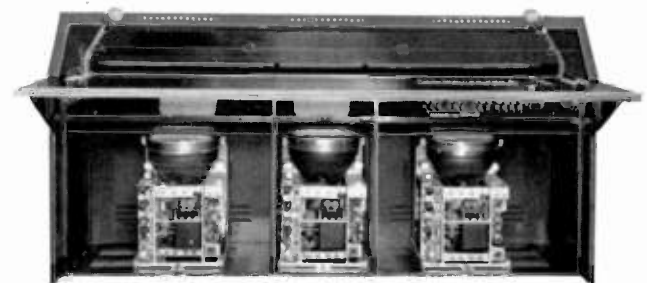
Program Monitors, TM-1A, shown installed in Program Director's Console
