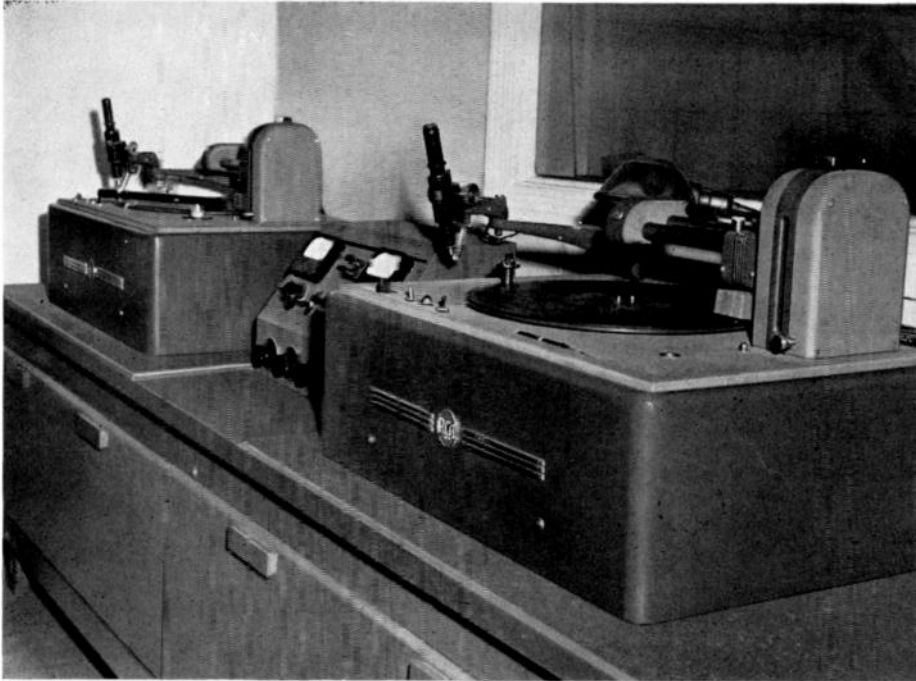
◆ Studio recording installation at KUTA, Salt Lake City, Utah, showing two bench-mounted RCA 73-B Professional Recorders.
