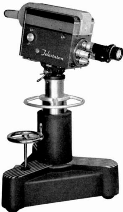
Studio type camera mounted on the pedestal.
