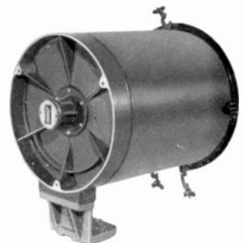
Transmitter, front end, showing Wave Guide Stub and Antenna Mounting Studs
