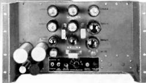
Regulated Power Supply, 580-C. Output adjustable between 260 and 295 volts—at 50 to 400 ma. Less than 0.25-volt variation between min. and max. load. Includes meter selector switch and meter jack.
