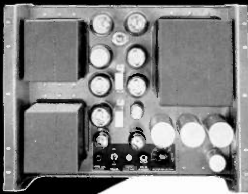
Regulated Power Supply (Heavy-Duty) WP-33B. Provides well-regulated d-c voltage at loads of 200 to 600 ma. Adjustable output, 260 to 295 volts. Voltage variation, less than 0.2 volt between minimum and maximum load.
