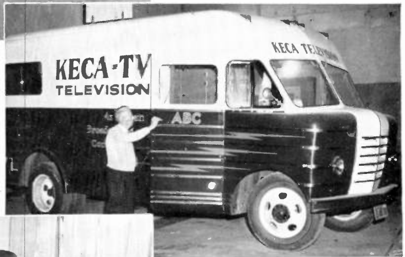
KECA-TV. KECA-TV's television field truck—like many other TV stations—is an RCA "studio on wheels." It is complete with RCA image orthicon cameras, camera tripods, camera control units, on-the-air master monitor, camera switching system, sync generator, microwave relay equipment, power supplies. KECA-TV also uses RCA studio cameras, film equipment, turntables, microphones, and an RCA Superturnstile antenna.
