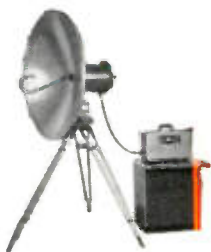
RCA Microwave Relay Transmitter TTR-1A. Transmits the picture signals from field to studio (or from studio to transmitter). It includes a parabolic antenna with hook-shaped wave guide, built-in transmitter, and remote control unit. Matching receiver unit at the station picks up the microwave relay signal.
