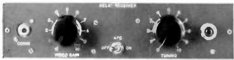
Relay Receiver Control, MI-26247. Controls video gain and receiver tuning. Includes 2 potentiometers, AFC "on-off" switch, tally light, and telephone jack.
