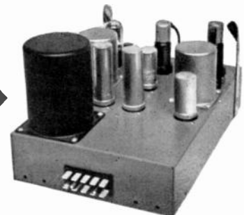
BA-2C Amplifier—Rear view. Plug-in chassis permits easy removal of amplifier for servicing
