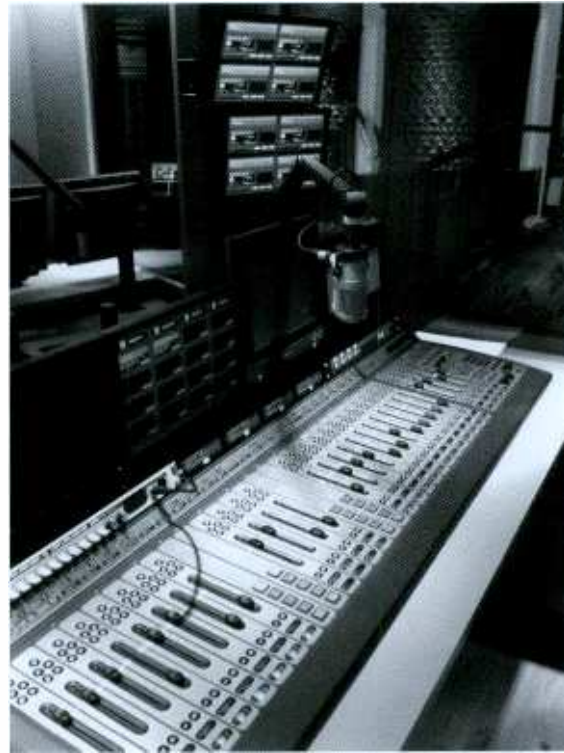
World's largest AoIP mixing console? Likely. This 36-position, 28-fader Axia Element is in the master control room of NRJ Networks, Paris.
