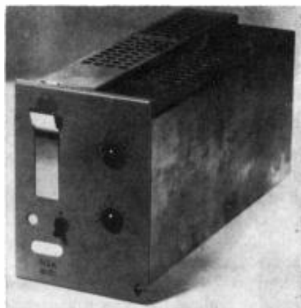
Neumann NSK Plug-in Power Supply unit for the Model SM-2 Stereo Microphone showing the two separate remote controls for changing the directional pattern of each of its two microphone capsules.
