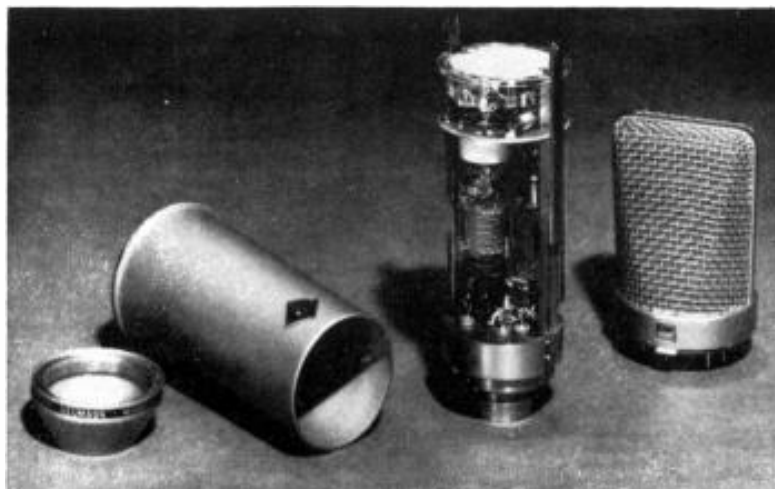
Neumann U-67 Condenser Microphone — shown disassembled into its amplifier, capsule head plug-in unit, housing and fastening ring. The M-269 Model version of this same unit is equipped with remote controlled directional characteristic.
