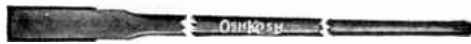
Handles made from hard rock maple. Tamping head faced with an iron shoe.
