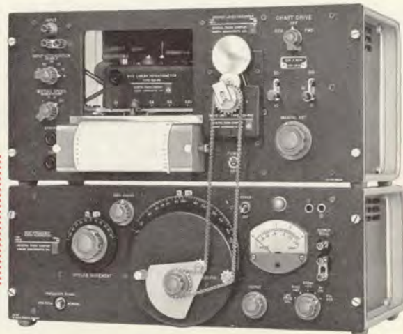
Type 1304-B Beat-Frequency Audio Generator driven by a Type 908-R96 Dial Drive, for use with an XY plotter.
