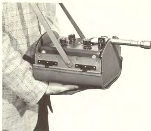
The sound-level meter is here operated while in its leather carrying case, with the microphone in the horizontal operating position.
