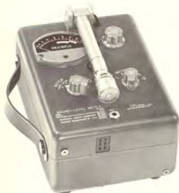
The Type 1551-C Sound-Level Meter with the microphone in the storage position and batteries automatically disconnected.
