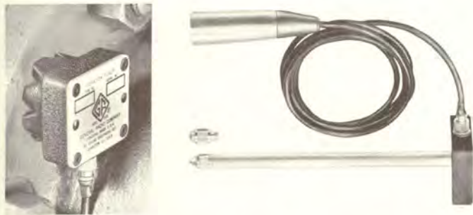
(Left) Vibration pickup with permanent-magnet clamp. (Right) Vibration pickup with probe and tips.
