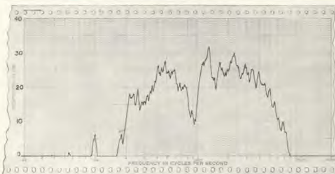
Plot of frequency response of a public-address system made on the graphic level recorder driving the frequency dial of the beat-frequency audio generator.
