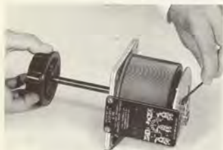
Shaft can be easily adjusted or replaced without disturbing other parts of the assembly.
