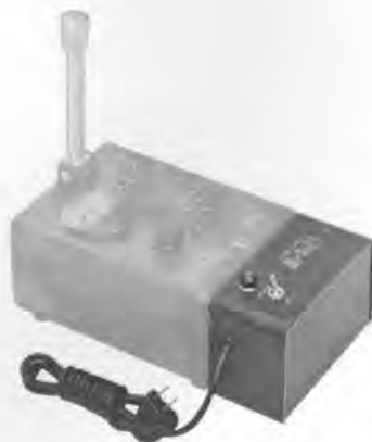
The Type 1551-C Sound-Level Meter can be ac-operated by means of the Type 1262-B Power Supply, which plugs directly into the base of the Sound-Level Meter.
