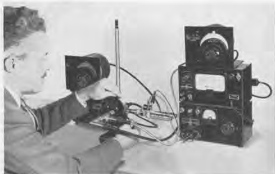
Admittance Meter set up for VSWR measurements on a coaxial switch.
