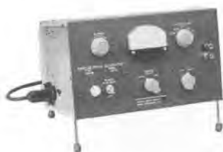
Extendible legs permit a tilted position (left); panel extensions (right) adapt the instrument for relay-rack mounting.
