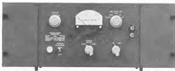
Extendible legs permit a tilted position (left); panel extensions (right) adapt the instrument for relay-rack mounting.
