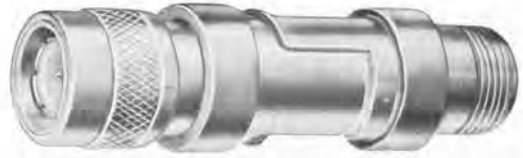
Type 874-QCP and -QNJA Adaptors plugged together. This assembly will connect a Type C jack to a Type N plug.
