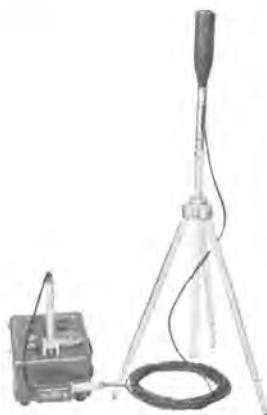
Transformer fastens to one end of Sound-Level Meter, and is connected in place of microphone, as shown.
