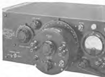
Motor drive attached to a 908-type dial on the Type 1304-B Beat-Frequency Audio Generator.
