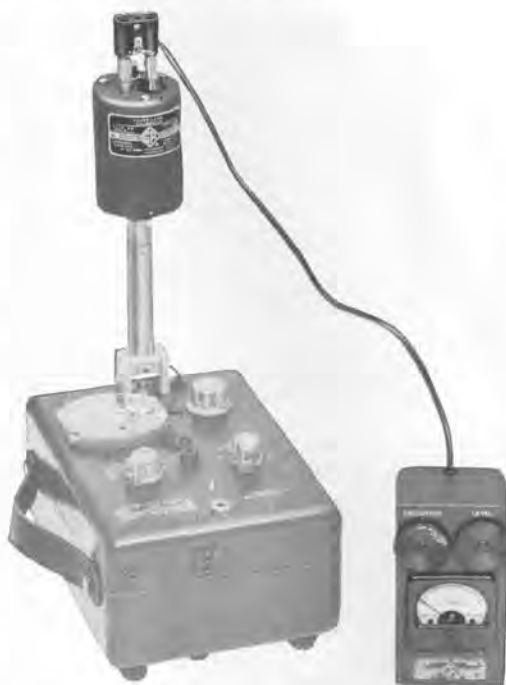
Calibrator fits over Microphone of Type 1551-C Sound-Level Meter. At right is Type 1307-A Transistor Oscillator.
