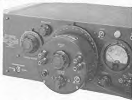
Type 1304-B Generator driven by a Type 908-R Dial Drive, for use with an X-Y plotter.
