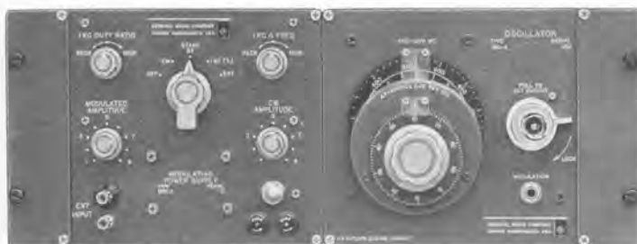
Type 1264-A Modulating Power Supply assembled with a Type 1361-A Oscillator and Type 480-P416 Panel Extensions for relay-rack mounting.
