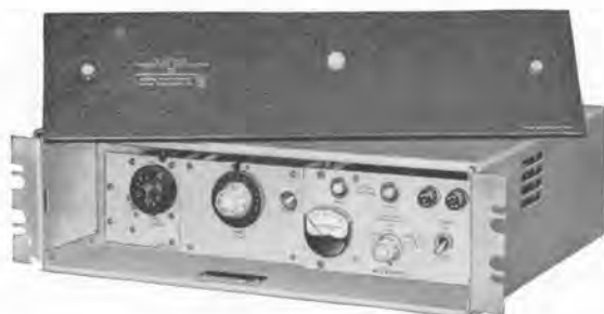
View of Type 1113-A Standard-Frequency Oscillator control panel. The front panel is held in place with two catches, and is easily removed for adjustment of controls or observation of oven performance.
