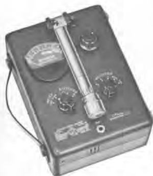
The Type 1551-C Sound-Level Meter with the microphone in the storage position, and batteries automatically disconnected.
