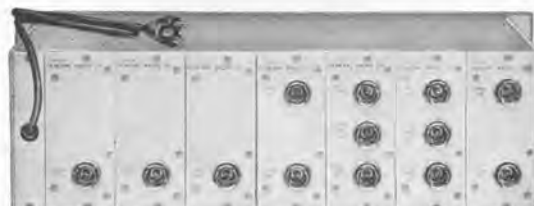
Rear view of the frequency divider, showing the plug-in units.
