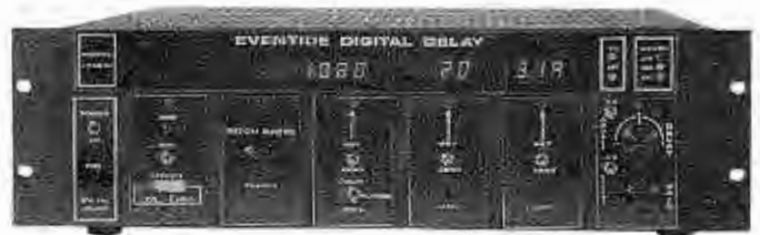
MODEL 1745M DIGITAL AUDIO DELAY LINE (320 ms delay, two outputs)
