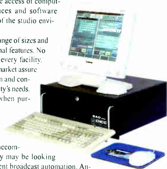
Enco Systems' DADpro32 Digital Audio Delivery System provides powerful production recording, editing, on-air reproduction and management, and interfaces to scheduling and billing systems. It can be used for both live-assist and automated operations.
