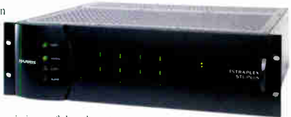
The Harris/Intraplex STL PLUS, when equipped with the OPX (Off-Premise Extension) option package lets you connect a telephone at the transmitter site to the PBX at the studio, just as if it were a local extension.
