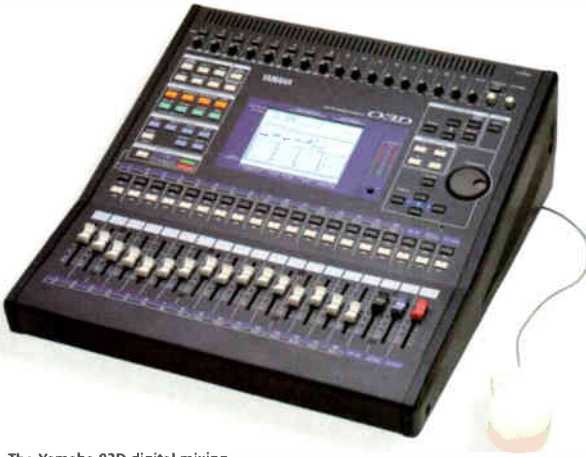
The Yamaha 03D digital mixing console is equipped with 18 analog and eight digital inputs, 32-bit signal processing, and over 300 factory-preset and user-definable libraries for effects, dynamics and other audio characteristics.
