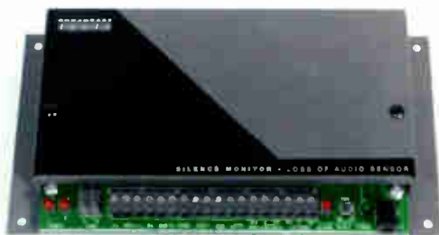
The Harris/Intraplex OutBack (bottom) ISDN codec and the Silence Monitor (top) made by Broadcast Tools can be combined to create a reliable backup for a station's STL. An absence of audio will close a relay in the Silence Monitor and switch the audio feed to a backup link via the OutBack codec and ISDN line.
