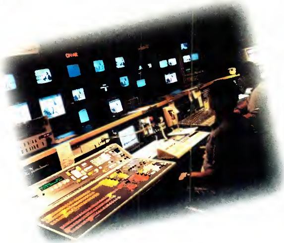
Three-channel automated master control system, News Channel 8 (Allnewsco) regional cable network, Springfield, Virginia
