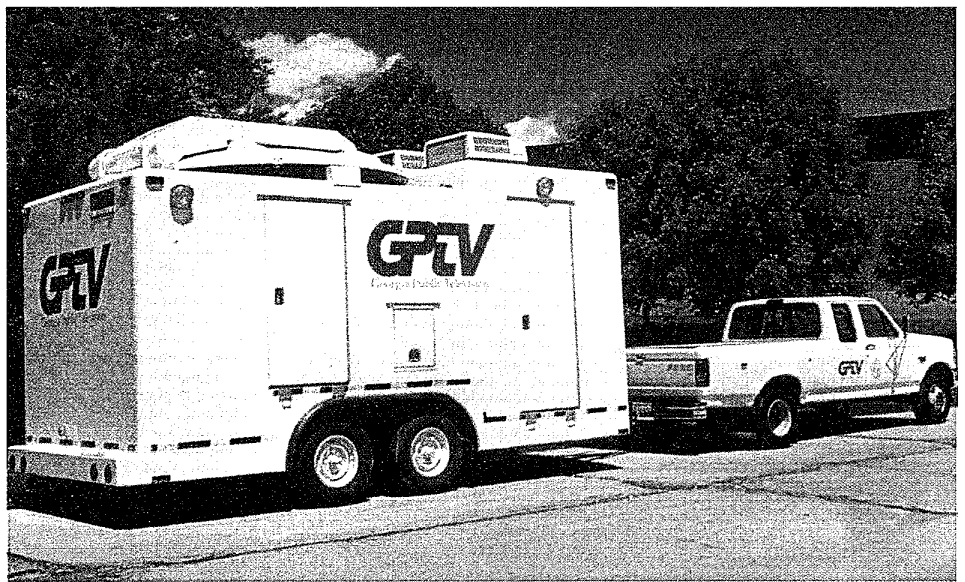
A unique trailerized satellite uplink system, the Harris S-20T is designed to be parked for days--or even weeks--on end. The tow vehicle provides ready local ground transportation for on-site crew.
