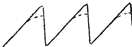
Fig. 7, Typical Waveform, Output V103 (V104 removed)
