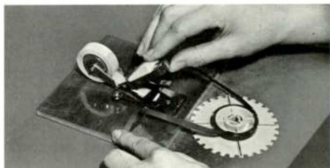
"Magnifying glass" attention is given to splicing tolerances to minimize "drop out" upon playback.
