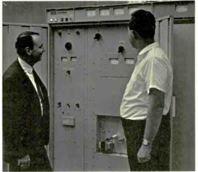
WGAN-FM, PORTLAND, MAINE —Utilizes a Gates 40 kW FM transmitter (two 20 kW transmitters with combiner and common exciter).
