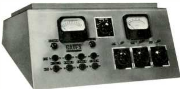
CCD-2 transmitter control console.
