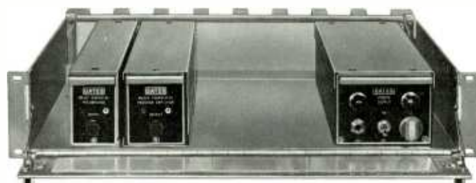
Above: M-6345 panel and shelf assembly, showing several "6300" series Solid-Statesman units. This assembly requires only 3½" x 19" of rack space.
