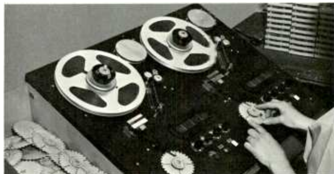
Tape is wound onto cartridge turntables with a precision tape winding machine to assure exact tape length and playing time.
