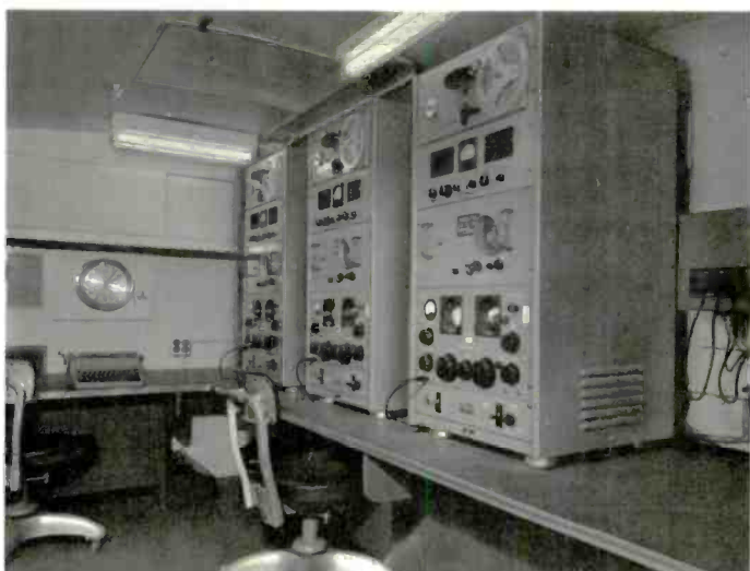
Mobile radio system designed and constructed by Gates for the Radio Bureau of the Republic of Korea provides complete medium and short wave broadcasting and public address facilities in a compact, specially designed van.
