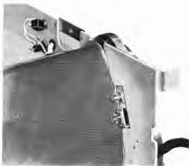
Through transparent slits in tape, special lamps and photocell arrangement control stop, cue and rewind of tape.
