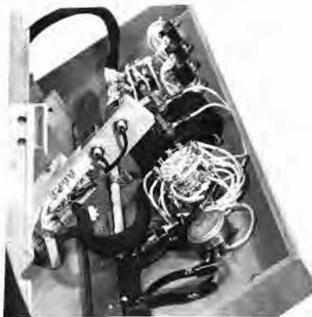
Back view of front panel showing how main components can be reached quickly and easily.
