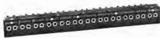
Above, PJ-343 jack panel has 24 jacks (12 pairs). Size: 1 1/2" x 19". Does not require jack mat. End brackets for rack mounting supplied.
