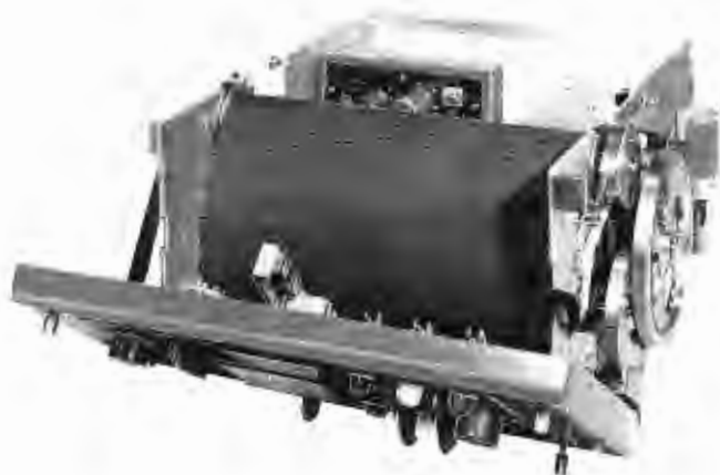
Front panel open and top off showing tape and amplifier. Top panel removes and front hinges down easily for complete accessibility to major components.
