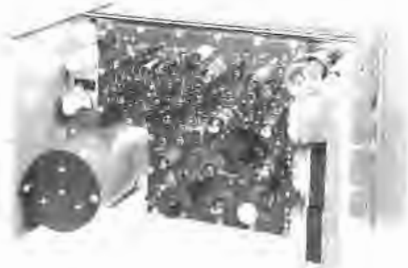
Rear view of M-4990 frequency monitor with dust cover removed. Each resistor and capacitor is firmly secured to the printed wiring chassis. Parts stacking is obviously absent.
