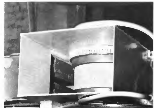
Fig. 9—Output cavity with one tuning plunger removed, showing ceramic and output coupling device.
