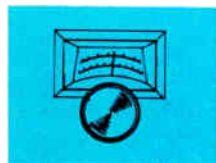
Position of hairline adjustable on panel, with cap to prevent accidental movement.
