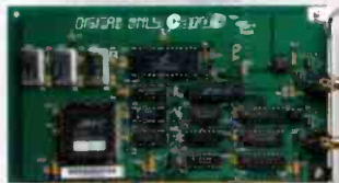
Digital Only CardD™ Stand-alone card for direct digital transfer to and from your DAT.
