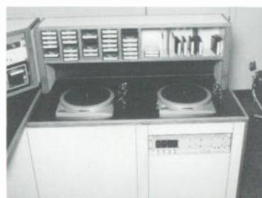
Locking the existing and new bases together and adding an overbridge creates a single integrated unit.
