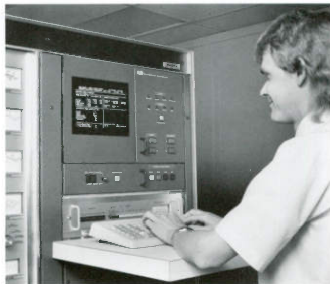
The optional Microprocessor Video Diagnostic System provides operational status, transmitter control and fault condition reports on a video display. A remote control package is available as an option to the system.
