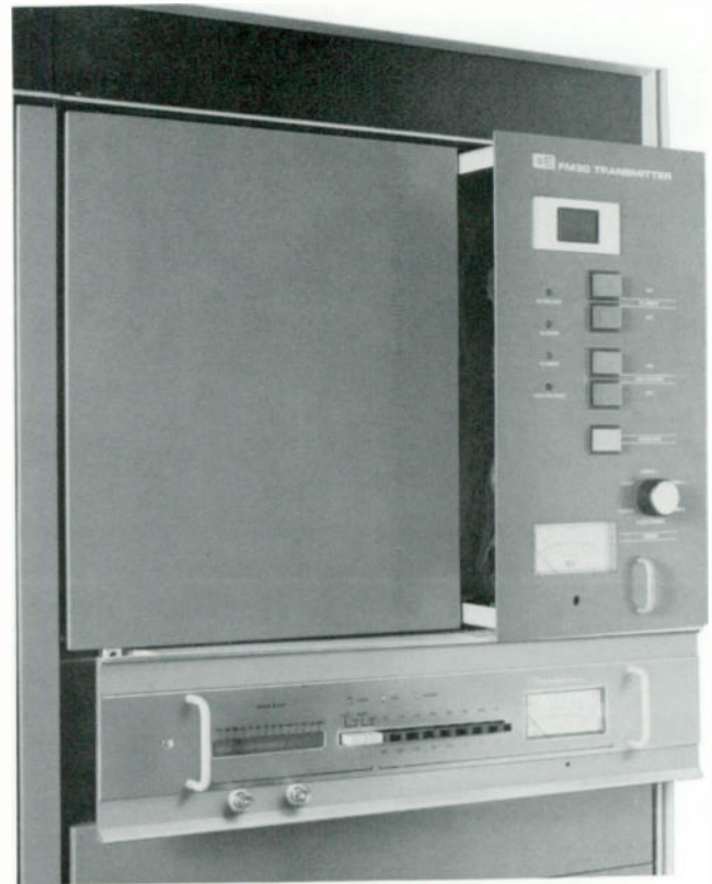
All transmitter control and status functions in the FM-30 transmitter are performed by a built-in digital controller (upper right part of photo). The advanced design Model FX-30 exciter is in the lower portion of the photo. Both units slide out for easy access.
