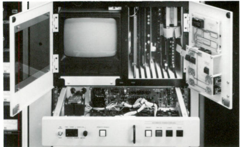
■ Transmitter Controller (shown with optional MVDS) and modular Automatic Power Control drawer pictured in the B/E FM-10B.
