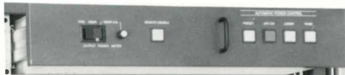
Close up view of the Automatic Power Control System (APC). This is one of three slide out modules in the FM-3.5A Transmitter.
