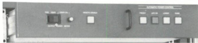
Close up view of the Automatic Power Control System (APC). This is one of three slide out modules in the FM-3.5A Transmitter.
