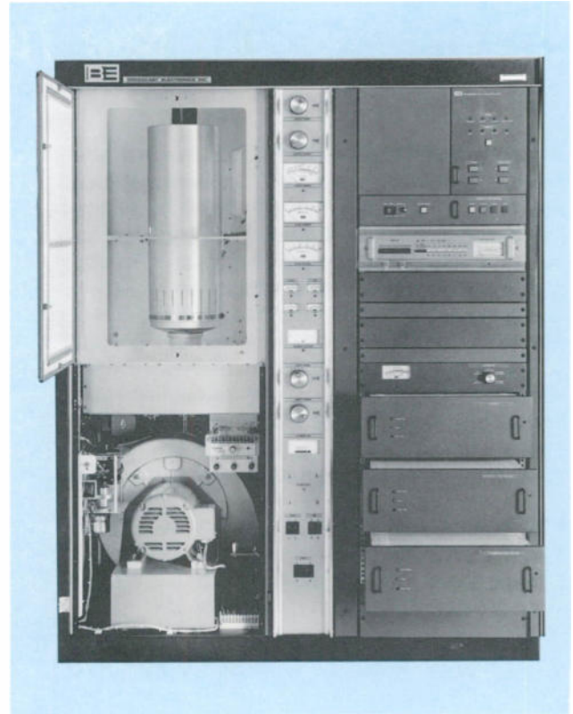
Front view of FM-35A with doors open and IPA drawers partially pulled out.
