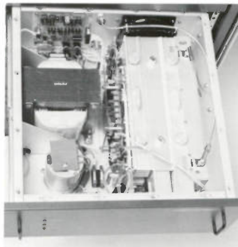
Slide out solid state IPA assembly includes power supply and can be used as a 250 watt transmitter.
