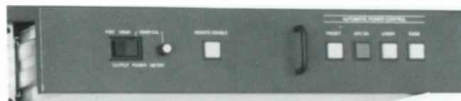
Close up view of the Automatic Power Control System (APC). This is one of four slide out modules in the FM-1.5A Transmitter.
