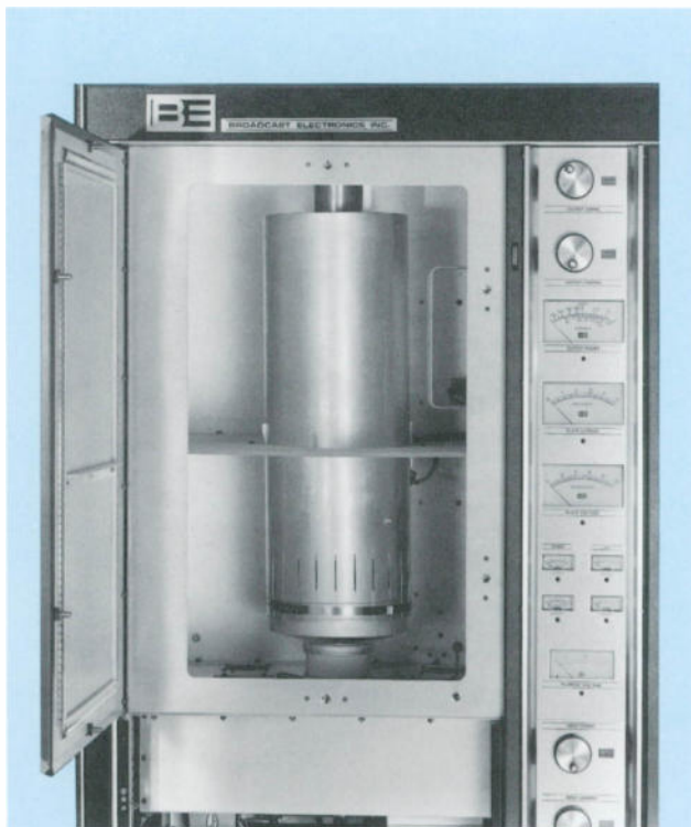
The Power Amplifier in the FM-35A transmitter employs a folded half-wave cavity, which eliminates the plate blocking capacitor and all sliding contacts in the output circuit.
