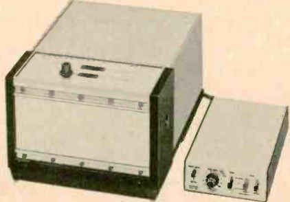
B EU-700 Monochromator. Wavelength range from 1900-10,000 Å, ±1 Å tracking accuracy, ±0.2Å reproducibility. Very low stray light. Resolves to better than 1 Å. EU-700, 70 lbs. ....$1275.00
