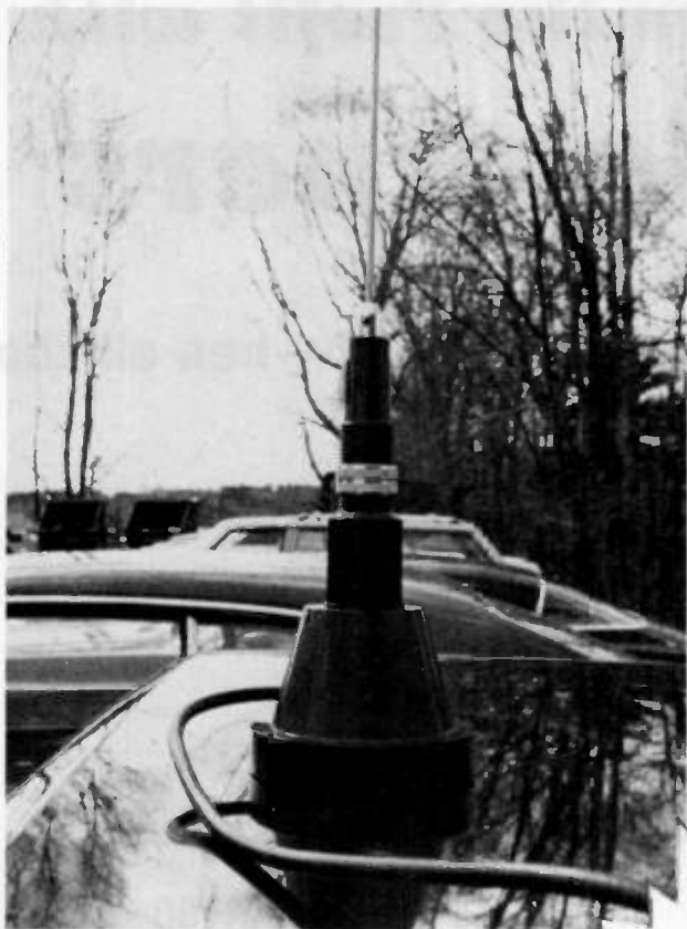
Two chromed tuning rings make tuning Lamtech's Bandit a lead pipe cinch. They vary the inductance of the antenna coil.
