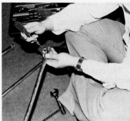
Putting the Wilson V-1 vertical together is a snap with its lengths of tubing. All it requires is inserting the tubes and tightening the clamps.
