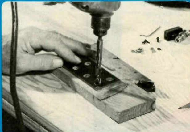
2. Seven holes are required in the back plate for the coax connector plugs—one master output and six accessory inputs.
