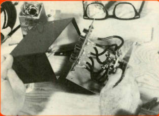
7. A metal lid is required to further shield the wires and plugs from any outside electrical interference. What may have seemed complicated in the beginning has turned out to be a very simple soldering project.
