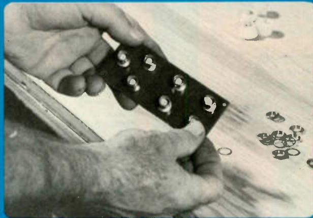
3. The single plug at the far left is the master output. A short length of coax cable connects this plug to the antenna input of your mobile or base transceiver.
