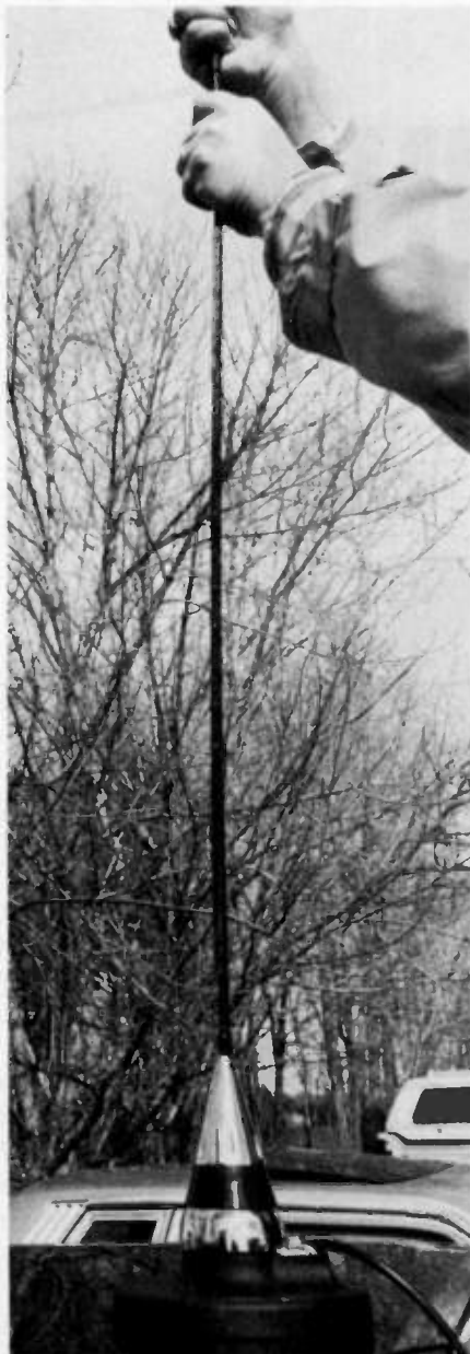
Tuning the American Antenna fiberglass stick is a matter of sliding a sleeve up and down to vary the capacitance (voltage) of the antenna.
