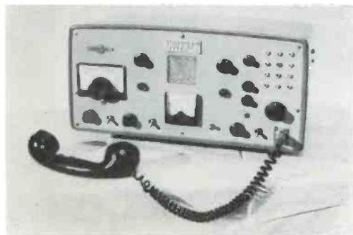
The Collins MBF in all its glory. Note that the rig has a telephone handset. If you want, you can forget the handset and use the set's loudspeaker for the microphone.
