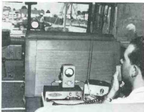
Engineer Joe Strawbridge calls an Amphenol mobile from Clark Cortez communications center during Friday's sedan race at Sebring. Amphenol 510-B was used to monitor Channels 1, 4, 8, 11, 13, 17 and 21, the channels used by the Renault Alpine, police, press, race officials and others around the track.
