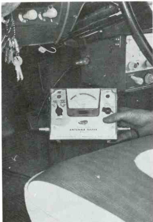
Fig. 4. Checking output and SWR with an in-line wattmeter (SECO).
