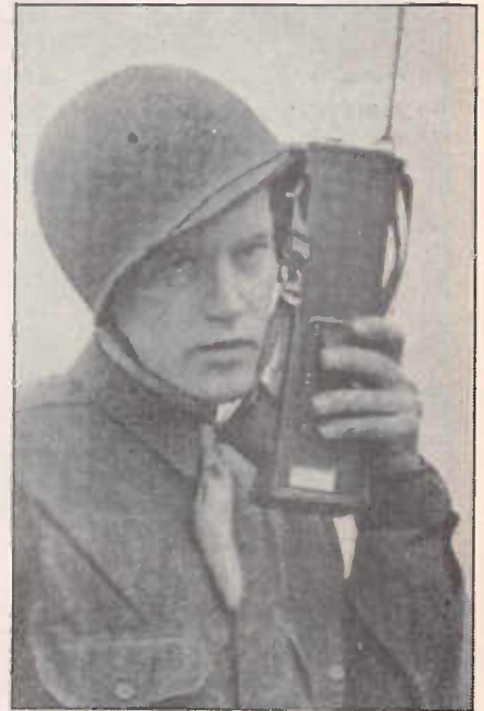
The true grand-daddy of CB radio – and American Army rig, about 14" long and with a handy send/receive switch on the side. Operated simply by extending the antenna, this rig weighed 5lb and had a 7 valve circuit
