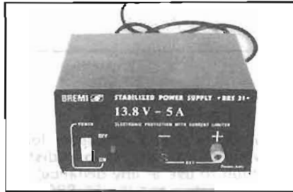
Bremi BRS 31 power supply unit
