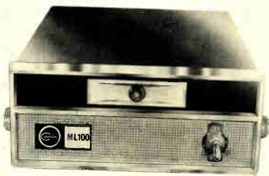
A transitional second generation boot, the e.c.i./courier ML-100 was actually on the way to being a full-blown third generation unit. It replaced the larger heat-generating model, and was fully transistorized—didn't require any "tune-up".
