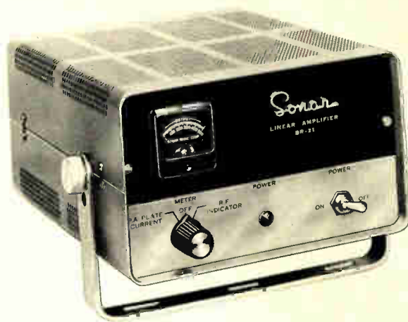
Sonar's BR-21 was another early entry into the second generation linear field. A panel meter gave you immediate information on what was happening inside. It provided a modest 14 watts boost.
