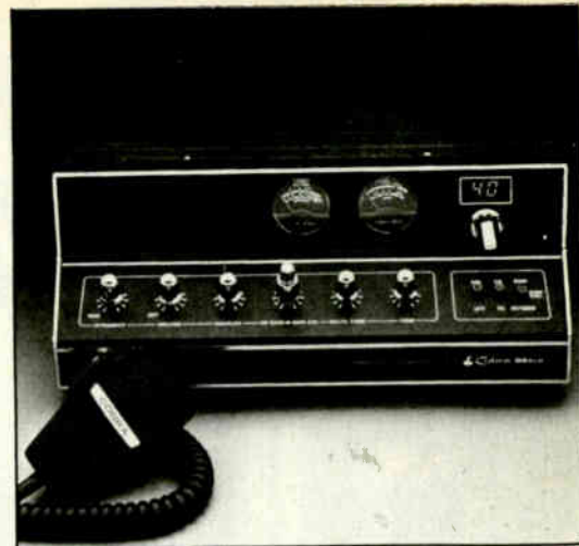
An impressive base station transceiver with built-in SWR meter. (Courtesy of Dynascan Corporation.)
