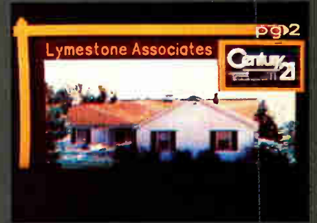
Channel 12 with channel 13 scrambled and with channel 4 decoding trap installed. Note that presence of decoding trap on converter exit channel has only slight effect on unscrambled channel 12.
