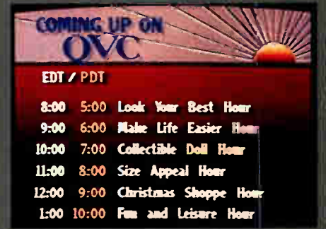
Channel 13 scrambled with positive RF encoder and unscrambled with channel 4 (converter exit channel) positive decoding trap. Note the absence of graininess even without pre-emphasis amplification.
